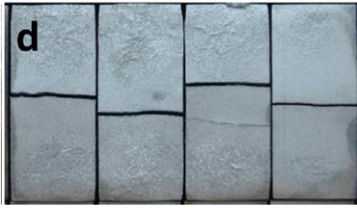
Figure 2 Deep cracking in the armour of an ITER divertor PFC mock-up following HHF test Typical taken from [Gavali[27]]
