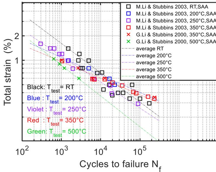
Fig. 4 Total strains versus number of cycles to failure of tests performed in UIUC [34, 35]
