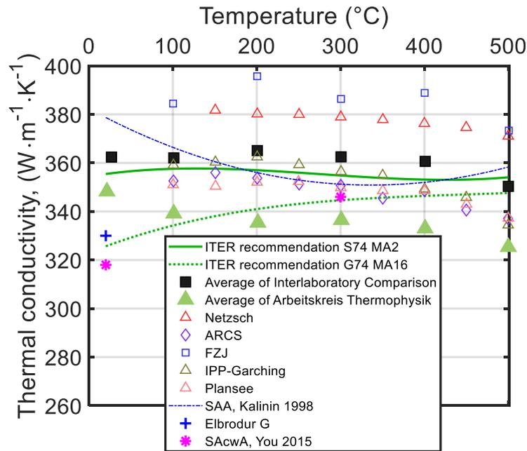
Fig. 7 Thermal conductivities versus temperatures. [1, 14, 29, 40, 42, 43]
