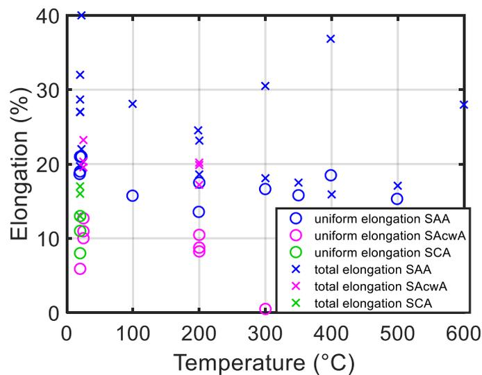
Fig. 3 Uniform and total elongations versus temperatures [1, 15, 26, 30-33]
