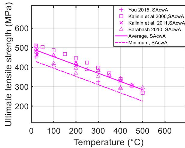
d) Ultimate tensile strengths of SAcwA specimens [1, 16, 30, 31]
