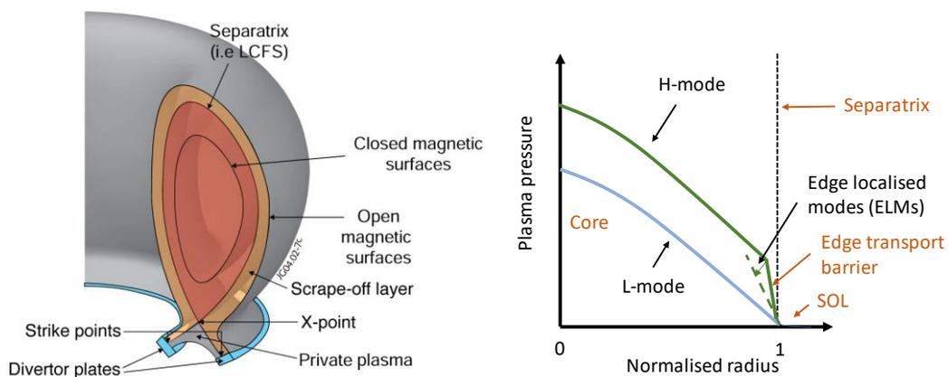
The left figure shows the geometry of the different regions of the tokamak. (Image credit: UKAEA) The right figure compares L-mode and H-mode pressure profiles in a tokamak plasma as a function of minor radius across flux surfaces from the centre of the plasma to the edge.
