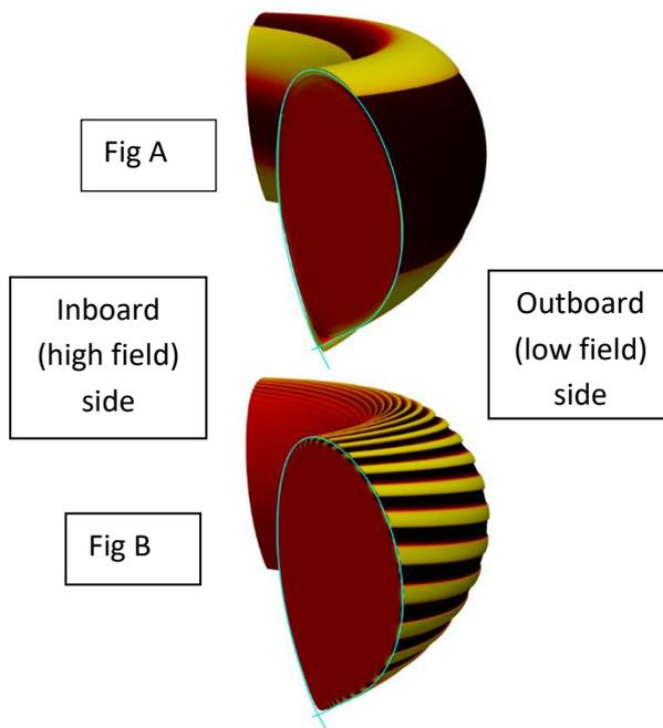
Figure-PB: The top plot shows a characteristic external kink mode; this is not only localised to the low field side, but also perturbs the inner, high field side of the flux surfaces. The bottom plot shows a characteristic ballooning mode displacement of a flux surface. The instability is aligned to the magnetic field and localised to the outboard or low magnetic field side of the tokamak.
