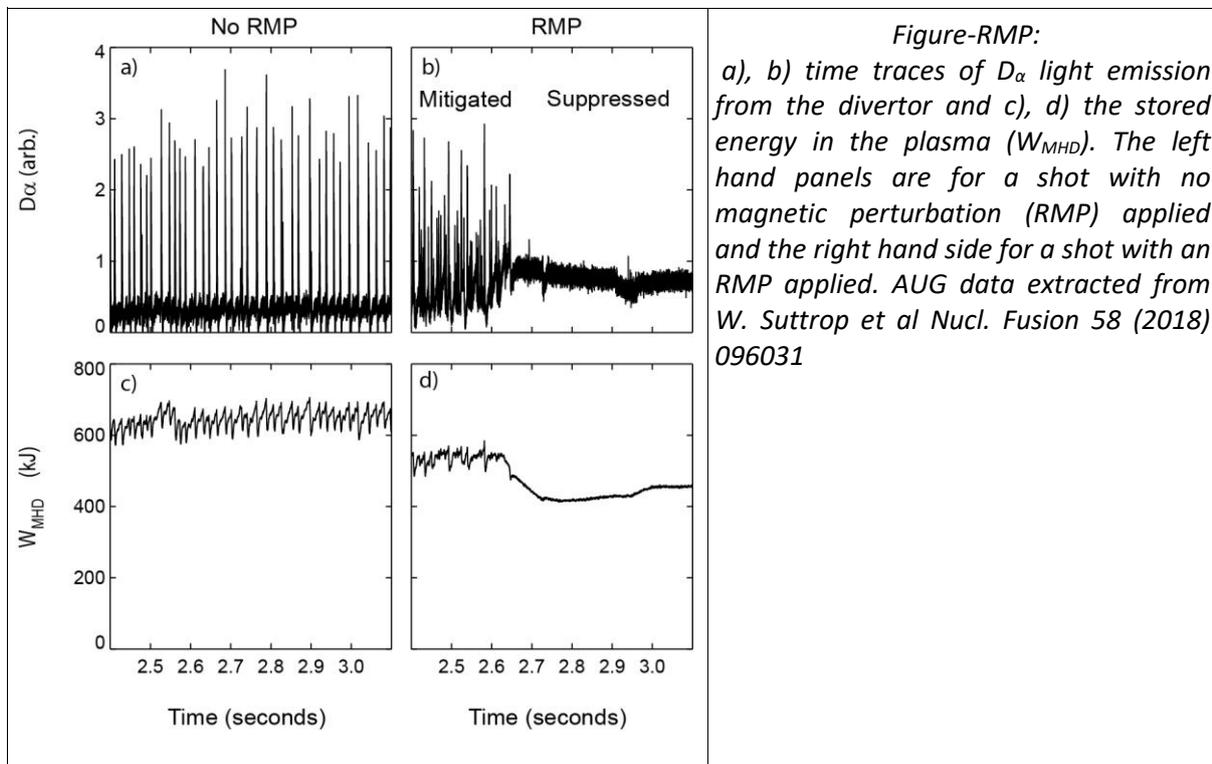
*Figure-RMP: a), b) time traces of  $D\alpha$  light emission from the divertor and c), d) the stored energy in the plasma ( $W_{MHD}$ ). The left hand panels are for a shot with no magnetic perturbation (RMP) applied and the right hand side for a shot with an RMP applied. AUG data extracted from W. Suttrop et al Nucl. Fusion 58 (2018) 096031*
