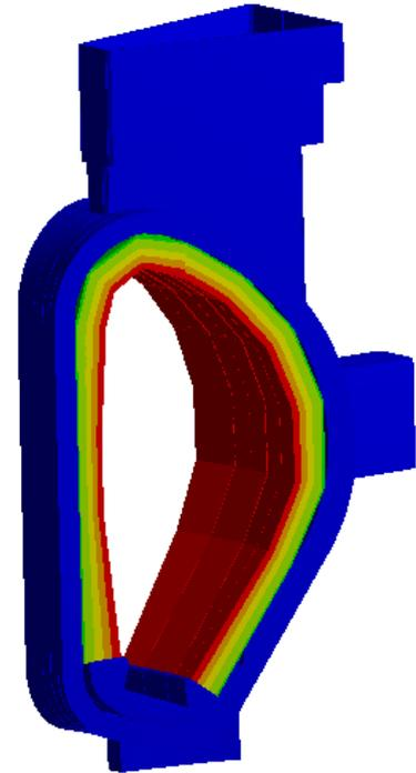
Figure 8.: Implemented temperature distribution for normal operation.
