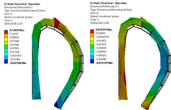
Figure.9.: Vertical and radial displacements during normal operation.
