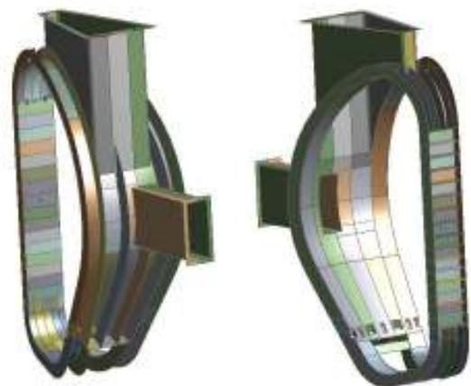
Figure.5. Vacuum vessel inner shell and stiffener ribs.
