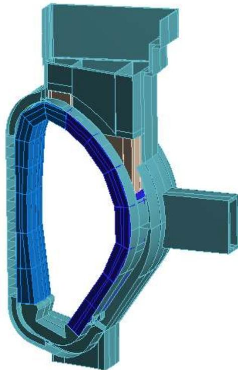
Figure.4. DEMO sector model with VV toroidal side removed to show internal ribs and upper port. Three upper port shield plugs (cyan) on top of five blanket segments (blue) with pipe connection locations "chimneys" (brown).
