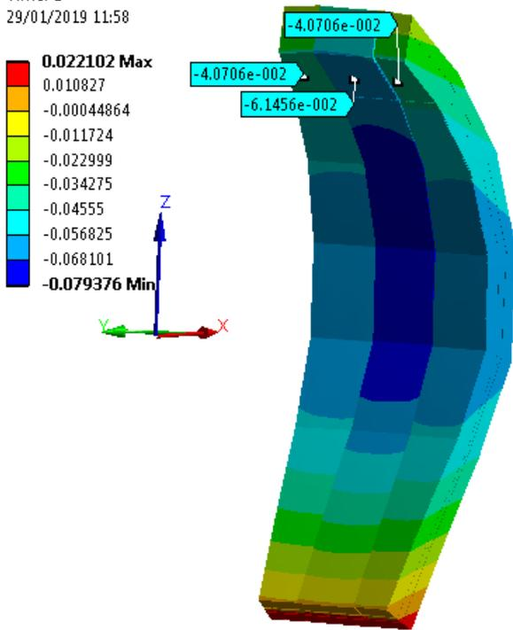
Figure.11.: Radial displacements during normal operation, with values at the top [m].
