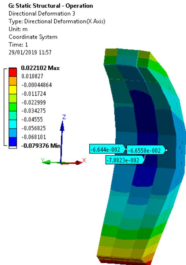
Figure.10.: Radial displacements during normal operation, with values at the centre [m].
