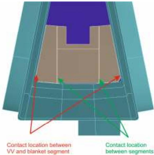
Figure.1. Toroidal support locations between the VV and lateral segments and the COB and lateral segments.
