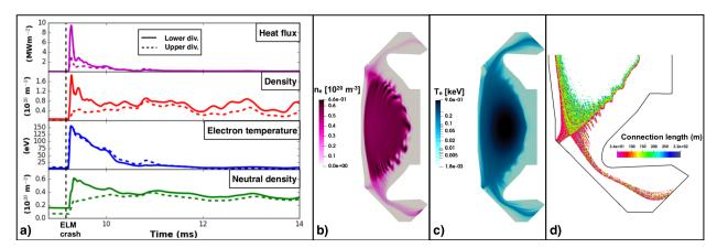
Figure 12: a) The evolution of the peak outer target values for the heat flux, density, electron temperature and neutral density for the upper (dashed lines) and lower (solid lines) divertors. A poloidal plot of the density b) and electron temperature c) during the ELM. d)Poincare plot of the magnetic field structure during the ELM.
