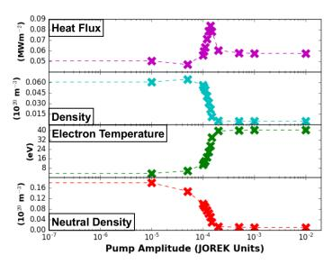
Figure 7: The saturated peak heat flux, density, electron temperature and neutral density on the outer lower divertor target as a function of pumping amplitude.
