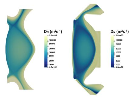
Figure 15: The amplitude of the diffusive neutral coefficient according to the calculation from Eq. 15, for the MAST L-mode case (left) and the MAST-U Super-X H-mode case (right).
