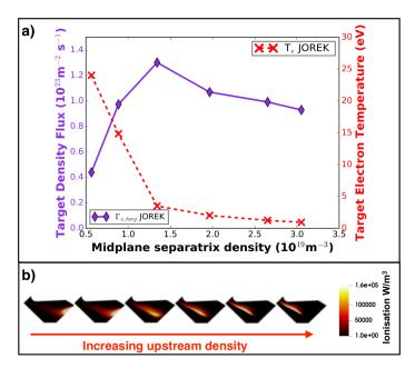
Figure 6: a) The target density flux and target electron temperature (at the separatrix) as a function of upstream density. b) The ionisation in the lower divertor is shown for the R4 scan from the JOREK simulations.
