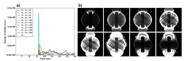
Figure 11: a) The evolution of the kinetic (coloured lines) and magnetic (grey lines) energy of the mode numbers for the multi-mode simulation. b) The evolution of the filamentary structures during the multi-mode ELM simulation imaged with a synthetic fast camera diagnostic.
