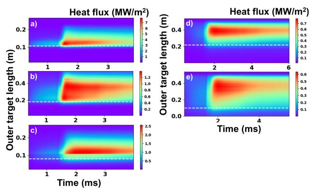
Figure 5: Heat flux patterns onto the outer target for R1-R5 shown in a)-e) respectively. The white dashed line indicates the position of the separatrix. Note the different length, time and heat flux scales in each heat flux pattern.
