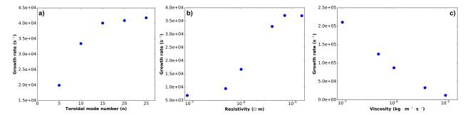
Figure 2: Linear growth rate of the instability as a function of a) toroidal mode number with a resistivity of  $5.4 \times 10^{-6} \Omega$  m and a dynamic viscosity of  $3.7 \times 10^{-6} \text{ kg.m}^{-1} \cdot \text{s}^{-1}$ . b) Resistivity scan with n = 20 and dynamic viscosity of  $1.5 \times 10^{-6} \text{ kg.m}^{-1} \cdot \text{s}^{-1}$ . c) Viscosity scan with n = 20 and a resistivity of  $1.0 \times 10^{-5} \Omega$  m.
