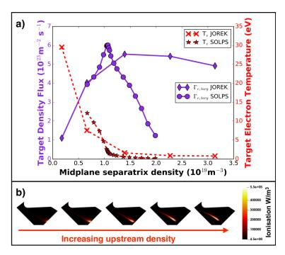
Figure 18: a) The target density flux and target electron temperature as a function of upstream density, comparing JOREK with SOLPS [16] for the R5 scan. b) The ionisation in the lower divertor is shown for the R5 scan from the JOREK simulations.
