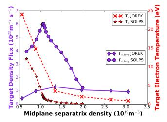
Figure 17: a) The target density flux and target electron temperature as a function of upstream density, comparing JOREK with SOLPS [16] for a R4 scan.
