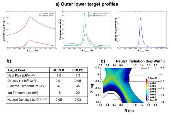
Figure 16: a) The plasma density and neutral density (left), electron and ion temperature (centre) and heat flux (right) as a function of major radius at the lower outer target. The black dashed line indicates the separatrix position. b) Table comparing JOREK and SOLPS peak outer target values. c) JOREK neutral line radiation in the lower divertor region, the white line indicates the separatrix.
