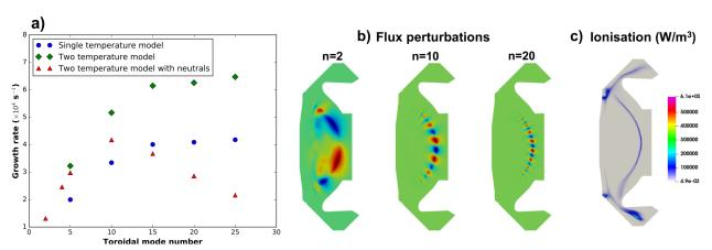
Figure 10: a) The growth rates as a function of toroidal mode number for the visco-resistive reduced MHD single temperature JOREK model, the two temperature model and the two temperature model with neutrals. b) The flux perturbations during the linear growth phase of the simulations for n=2 (left), n=10 (centre) and n=20 (right). c) The ionisation in the poloidal plane in the linear growth phase of the n=20 simulation.
