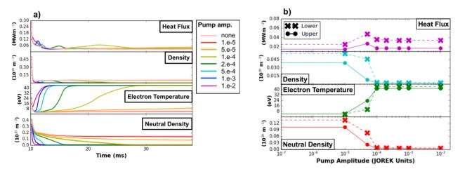
Figure 14: a) The evolution of the peak lower outer target heat flux, density, electron temperature and neutral density at different pumping amplitudes, after the ELM. b) The saturated peak target values, after the ELM, for the heat flux, plasma density, electron temperature and neutral density as a function of pumping amplitude for the upper and lower divertor targets.
