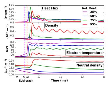
Figure 9: Evolution of peak outer target values for varying reflective coefficient starting at a reflectivity of 95% (red lines) and decreasing. The recovery to pre-ELM conditions is only observed at high reflectivity.
