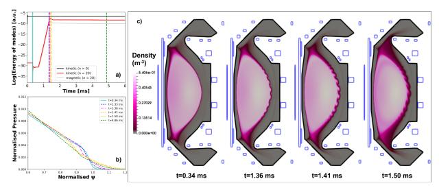
Figure 3: a) Evolution of the energy of the modes. b) The evolution of the pressure profile. c) Density filament evolution during the crash.
