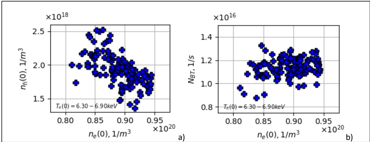
Figure 9: a) Central fast ions density,  $n_{fi}(0)$ , versus central electron density,  $n_e(0)$ , for JET's 3.3T/3.5MA high-performance baseline pulses; b) Total BT neutrons,  $N_{BT}$ , versus central electron density,  $n_e(0)$ . The subset of data is for central electron temperature in the range  $T_e(0)=6.3-6.9\text{keV}$ .
