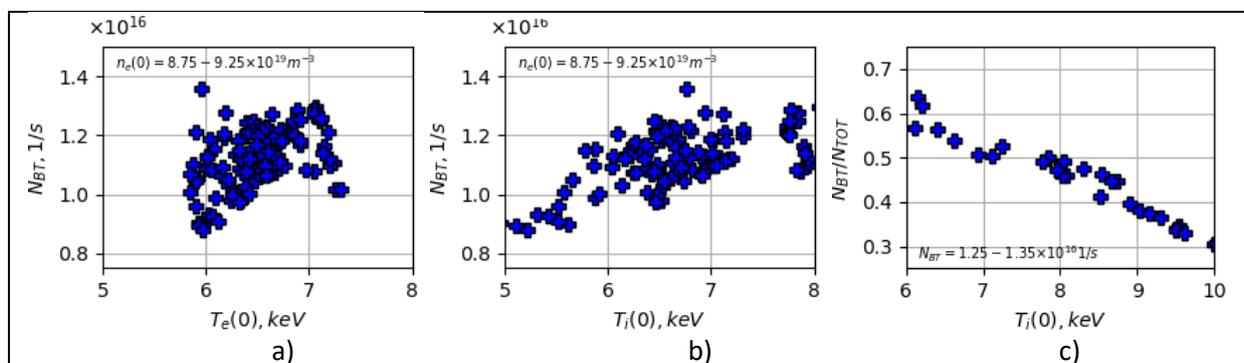
Figure 11: BT neutrons,  $N_{BT}$ , versus central electron  $T_e(0)$  a) and ion temperature  $T_i(0)$  b) for 3.3T/3.5MA baseline pulses with  $n_e(0)=8.75-9.25 \times 10^{19} \text{ m}^{-3}$  and the ratio of BT neutrons to total calculated neutrons,  $N_{BT}/N_{TOT}$ , for  $N_{BT} \approx 1.3 \times 10^{16} \text{ 1/s}$  in c)
