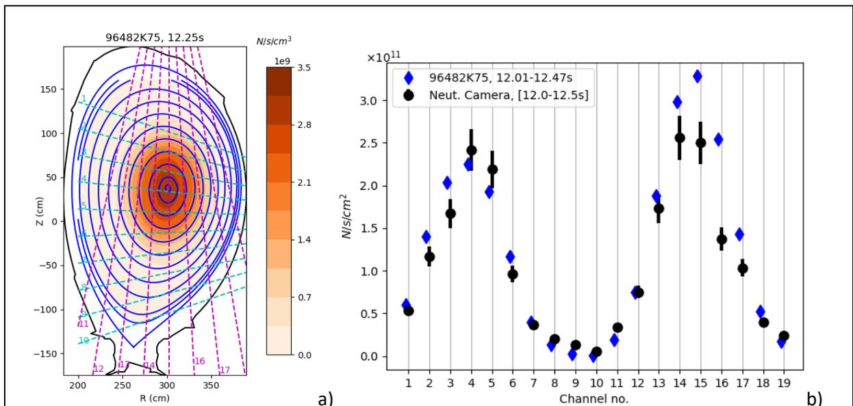
Figure 5: a) Neutron camera lines of sights for 10 horizontal and 9 vertical channels. Provided is the plasma equilibrium and calculated neutron rates,  $R_{TOT}(R,Z)$  in  $1/s/cm^3$ , colour mapped in plasma cross-section for 96482K75, 12.25s. b) Neutron camera data for lines 1 to 19 (black) for pulse
