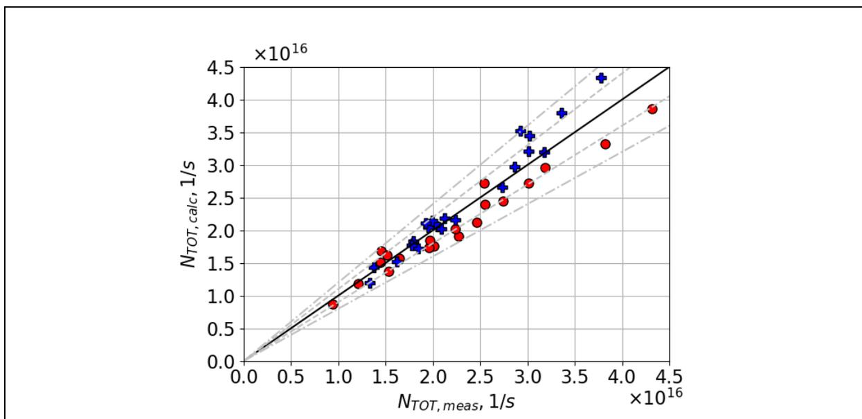
Figure 2: Calculated  $N_{TOT,calc}$  vs. measured  $N_{TOT,meas}$  total neutron counts for all recent JET high performance pulses. Baseline pulses are in blue crosses, whilst hybrid pulses are in red circles. The deviation of the calculated data from the measurements by 10% and 20% are shown by grey dashed and dash-dotted lines respectively.
