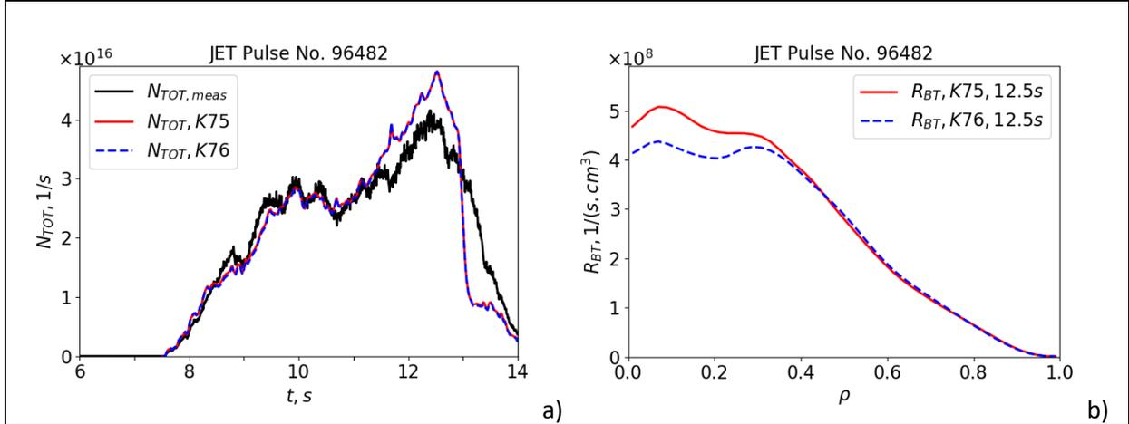
Figure 13: Total neutron count  $N_{TOT}$  in a) and BT neutron rates  $R_{BT}$  at 12.5s in b) for JET pulse #96482 modelled by TRANSP with RF power and RF kick operator (red lines) and with RF kick operator turned off (blue dashed lines). Experimental total neutron count (black lines) is provided in a) for comparison.
