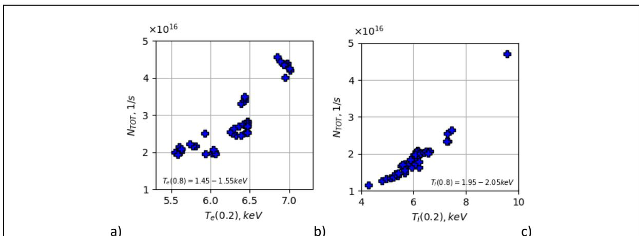
Figure 6: Total neutron counts as calculated by TRANSP,  $N_{TOT}$ , versus electron density a) electron temperature b) and ion temperature c) in the core at  $\rho=0.2$  for JET's high-performance 3.3T/3.5MA baseline pulses. The pedestal values, taken at  $\rho=0.8$ , are fixed and provided at the bottom of the graphs.
