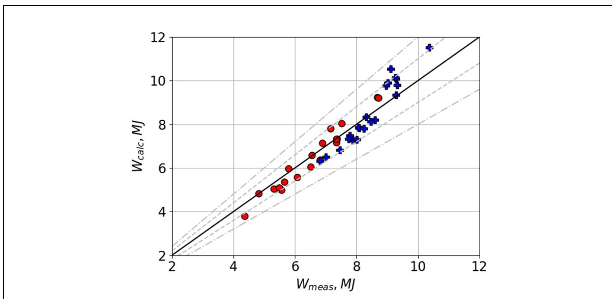
Figure 3: Calculated  $W_{calc}$  vs. measured via diamagnetic measurements  $W_{meas}$  plasma energy. Baseline pulses are in blue crosses, whilst hybrid pulses are in red circles. The deviation of the calculated data from the measurements by 10% and 20% are shown by grey dashed and dash-dotted lines respectively.
