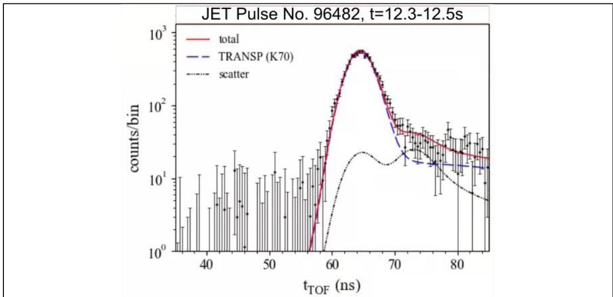
Figure 4: Neutron spectrum from TOFOR diagnostic for JET pulse #96482, 12.3-12.5s. Measured time-of-flight,  $t_{TOF}$ , (black points) is compared to total predicted (red) which is superposition of result from TRANSP fast ions distribution function (blue dashed line) and scattered neutrons (dash-dotted line).
