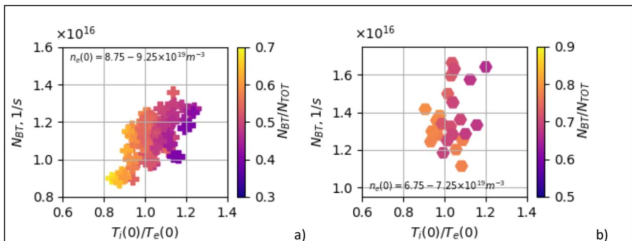
Figure 12: BT neutrons,  $N_{BT}$ , versus the ratio of central ion and electron temperatures  $T_i(0)/T_e(0)$  for 3.3T/3.5MA with  $n_e(0)=8.75-9.25 \times 10^{19} m^{-3}$  baseline pulses a) and 2.8-3.4T/2.15MA hybrid pulses with  $n_e(0)=6.75-7.25 \times 10^{19} m^{-3}$  b). Colour mapped symbols show ratio of BT neutrons to total calculated neutrons,  $N_{BT}/N_{TOT}$ .
