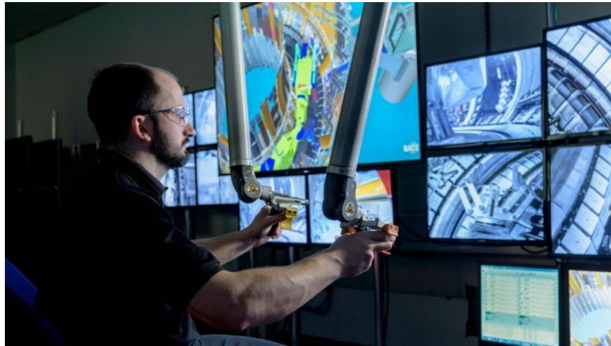
Figure 1: A remotely operated robotic facility, designed to maintain the Joint European Torus (JET) nuclear fusion experimental reactor.
