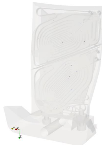
Figure 4. The 21 UM elements out of 1018163 (~0.002%) failing due to abnormal nuclear heating due to poor statistics.
