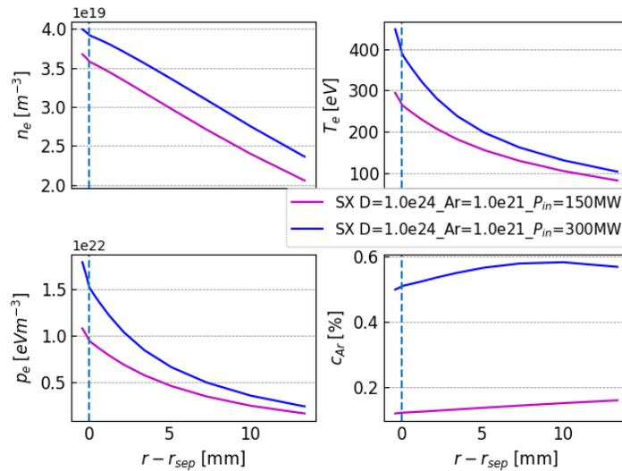
**Figure 6.** The radial profiles of electron density, temperature, static pressure and argon concentration at the outboard midplane in two DEMO SXD simulations with same deuterium fuelling and argon seeding rates at  $P_{in}=150$  MW and  $P_{in}=300$  MW.
