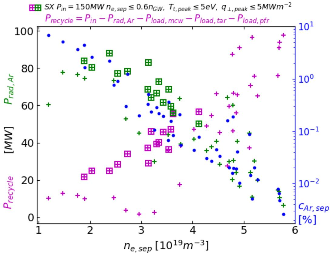
**Figure 8.** Radiated power by argon in the plasma,  $P_{rad,Ar}$  (green), the power available for ionizing deuterium neutrals,  $P_{recycle}$  (magenta), and the average argon concentration in the divertor region within the radial range of  $\lambda_q$  (blue), as a function of the OMP separatrix density, for DEMO SXD at  $P_{in}=150$  MW. The simulations within the operational space are marked with square symbols.
