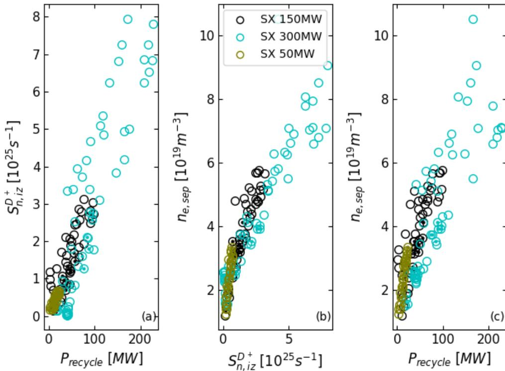
**Figure 9.** The correlation between  $P_{recycle}$  and  $S_n^{D+}$ ,  $S_n^{D+}$  and  $n_e$ ,  $P_{recycle}$  and  $n_e$  for the SXD simulations with low (50 MW), standard (150 MW) and high (300 MW) power input.  $P_{recycle}$  is the power available for ionizing the D neutrals, as defined in figure 8.  $S_n^{D+}$  is the ionization particle source of  $D^+$ .  $n_e$  is the density at OMP separatrix.
