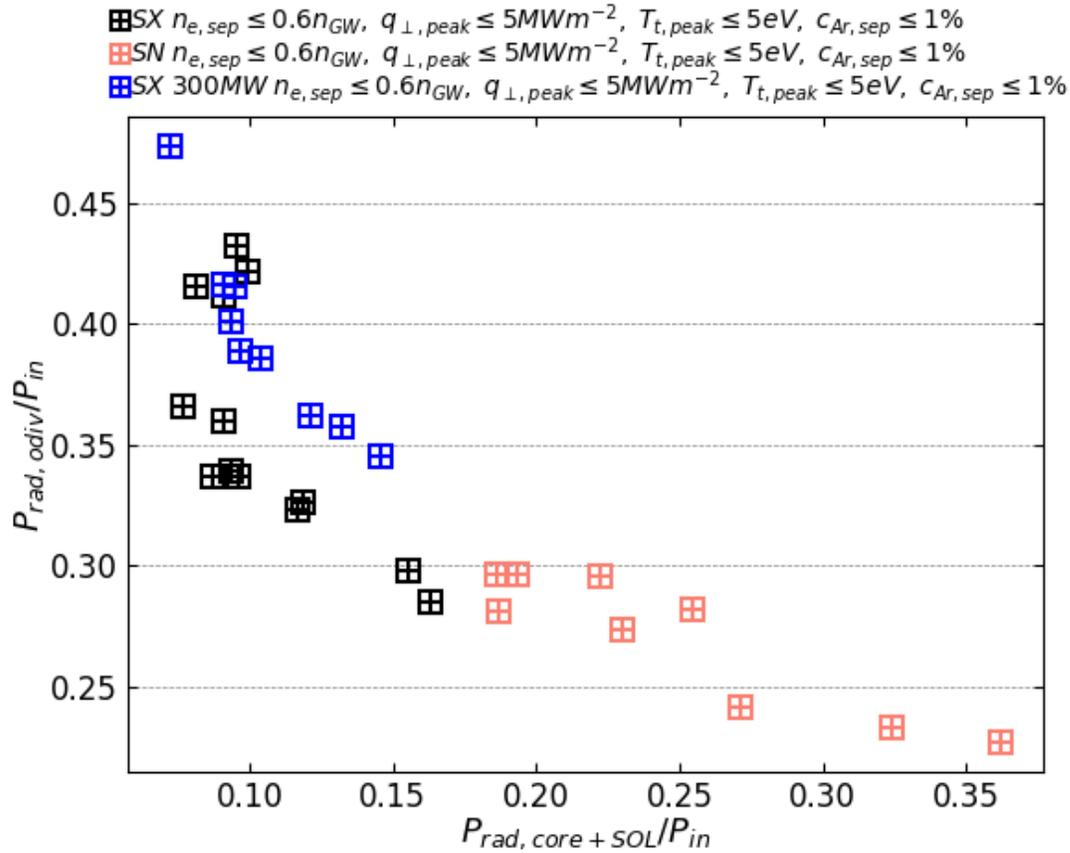
**Figure 4.** The radiated power in the outer divertor as a function of the fractional radiated power from the 'core' and SOL region (see definition in figure 1) above the X-point, both as fraction of the input power  $P_{in}$ . Only the simulations within the operational space are shown here for DEMO SXD at  $P_{in}=150$  MW and  $P_{in}=300$  MW, and SND at  $P_{in}=150$  MW.
