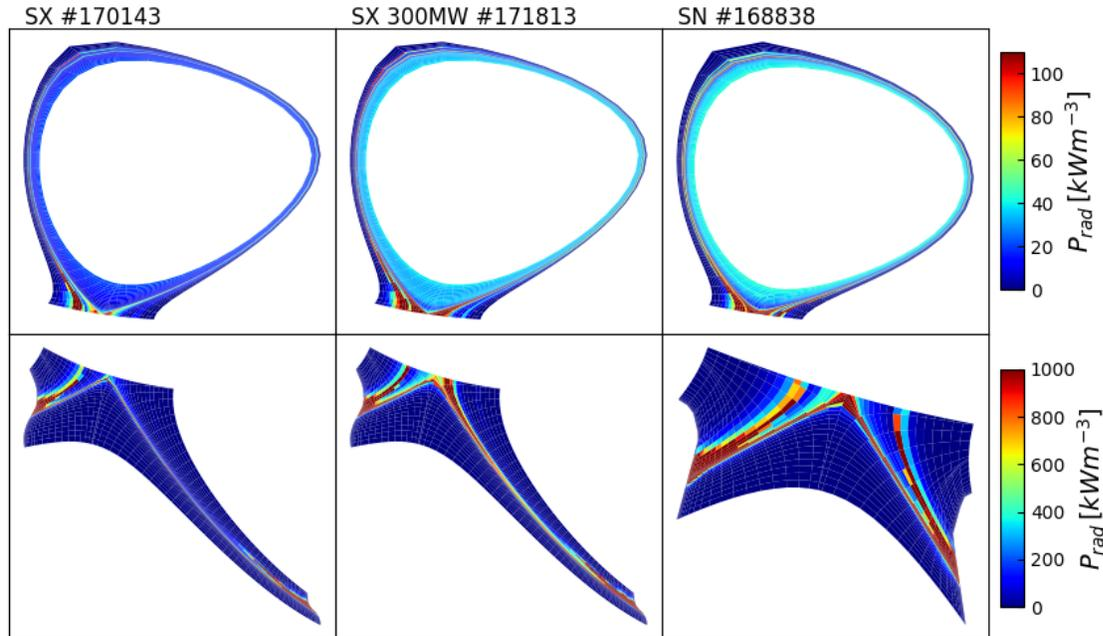
**Figure 5.** The total radiated power density distribution in the modelling domain for 3 selected simulations outline by the grey ellipse in figure 2, which are simulations within the operational space with similar upstream density. The upper row shows the radiation density distribution in the regions above the X-point, i.e. in the 'core' and SOL. The lower row shows the radiation density distribution in the divertor region.
