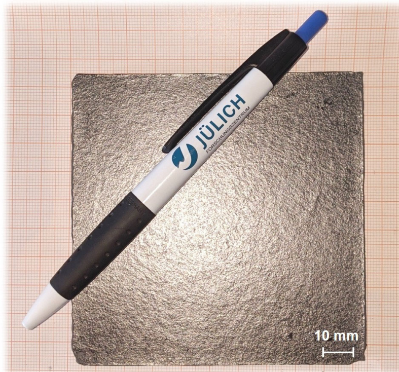
Figure 5. A large-scale bulk SMART alloy sample sintered using the industrial FAST facility.
