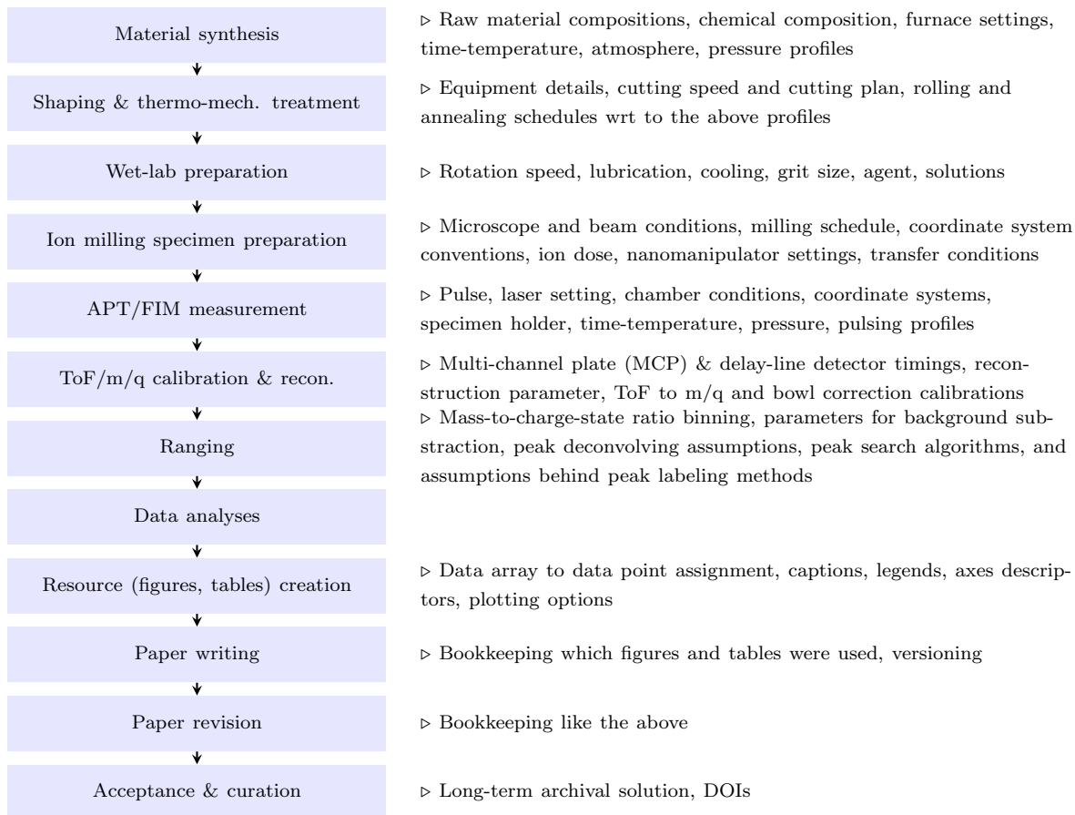
Figure 1: To the left: Key steps of one type of scientific workflow via which many APT/FIM specimens find entry into publications. To the right, an associated (incomplete) list of exemplary (meta)data which experimentalists ideally need to keep track of during each step.
