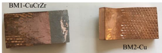
Fig. 18.- Sheared test on CuCrZr-Cu specimen brazed with NBLM™
