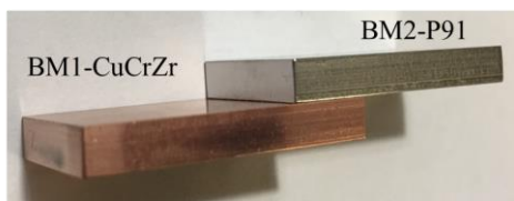
Fig. 19.- Poor-Acceptable wetting on CuCrZr-P91 specimen brazed with OB950™
