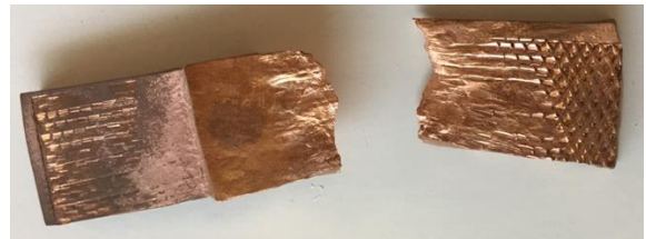
Fig. 20.- Sheared CuCrZr-Cu specimen brazed with OB1025™
