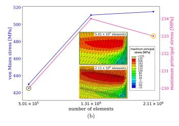
Figure 10. Variation of the von Mises and maximum principal stresses as functions of the total number of elements in an FEM model for (a) the initial design and (b) the modified design investigated in Sec. VII. Stresses are evaluated in the regions showed at higher magnification in figures 8 and 9. FEM mesh in these regions is shown here with a map of (a) the von Mises and (b) the maximum principal stress, to show the effect of two iterations of the mesh refinement algorithm.
