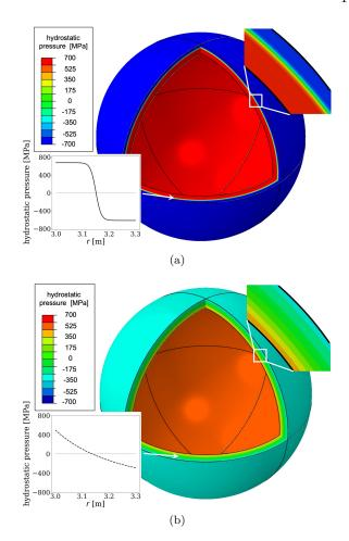
Figure 6. Contour plots of the hydrostatic pressure induced by irradiation corresponding to the profiles of densities of relaxation volumes of defects  $\omega(r)$  shown in Fig. 5a for case 1 in (a) and for case 2 in (b). The colour scale is the same in both plots, showing that stress is higher in case 1 than in case 2, despite the fact that the total relaxation volume of defects in the shell  $\Omega_{tot}$  is the same in both cases (see Fig. 5a).
