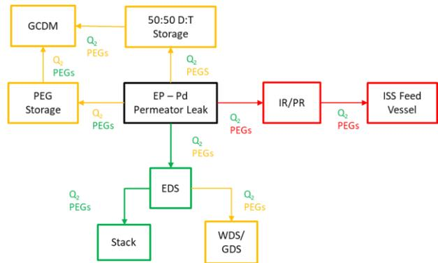
Figure 2: Traffic Light Representation of Flows following a Pd Membrane Break
