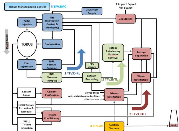
Figure 1: DEMO Tritium Fuel Cycle and Associated System Blocks, from [1].
