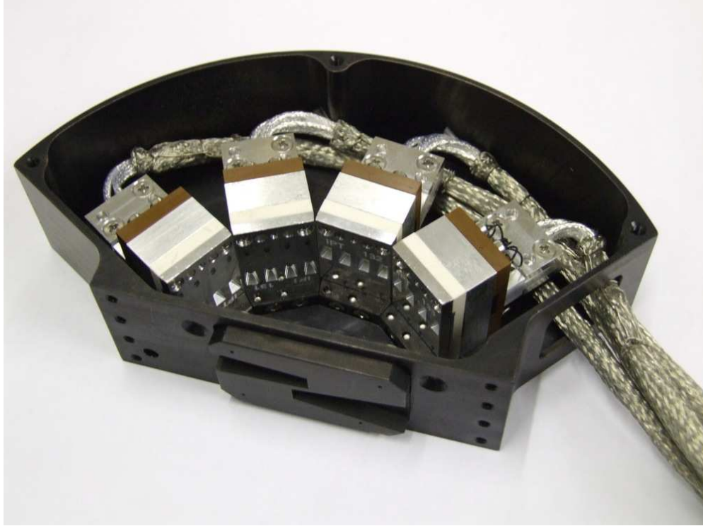
FIG. 2: Baffle-mounted bolometer camera, before installation. There are two apertures, each viewed by 2 4-channel sensors. A plate (not shown) sits between the apertures and sensors to prevent light from the wrong aperture reaching the sensor. The plate is ridged, and all the internal surfaces of the camera are blackened, to reduce internal reflections.
