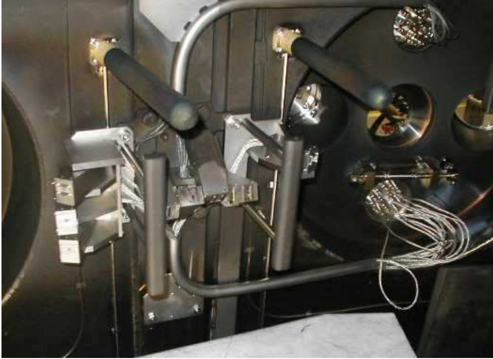
FIG. 1: The main chamber bolometer camera, as installed in MAST. Each 4-channel sensor is housed in a metal box. 3 sensors — 12 channels — provide a tangential view at the midplane in the same direction as the plasma current (seen on the left). 1 sensor — 4 channels — provides a tangential view in the opposite direction to the plasma current (right). 4 sensors in a 16-channel fan cover the poloidal cross section of the core plasma. For MAST Upgrade this same camera is used in the same location, but radially offset 10 cm from the wall.
