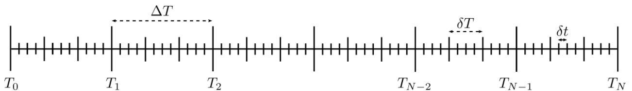
Figure 1: Schematic of the time domain decomposition. Three levels of temporal discretisation are shown: sub-intervals (size \Delta T ), coarse intervals (size \delta T ), and fine intervals (size \delta t ). Note how the discretisations align with one another and that \delta t \ll \delta T \leq \Delta T in our implementation.
