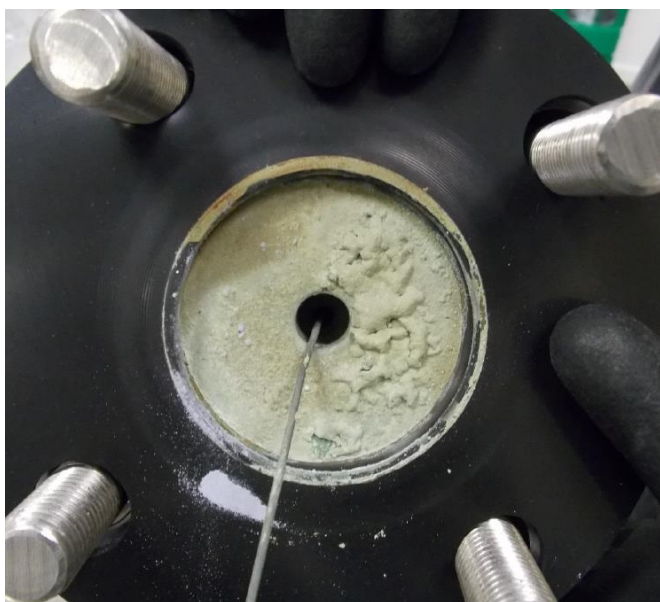
Figure 20 - thin layer of deposit on bottom flange following chronic HF/HCl mix test with Loflosorb
