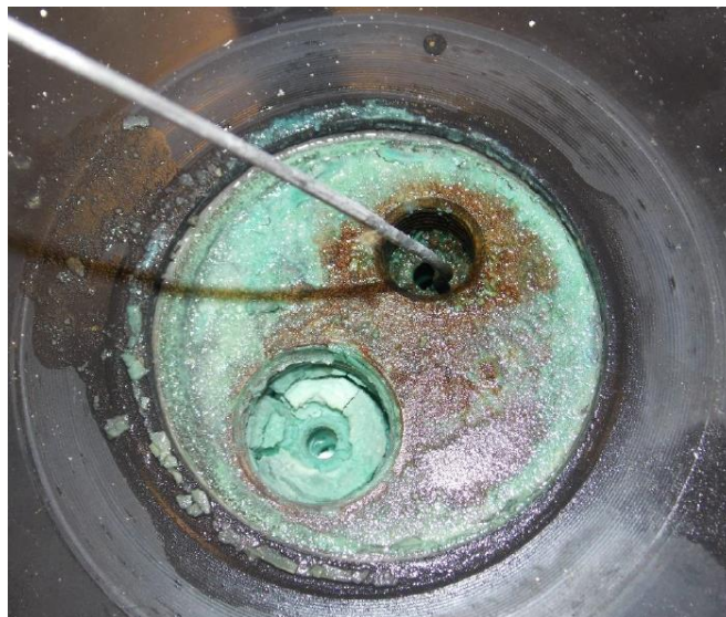
Figure 14 - corrosion product build-up on bottom flange and inlet pipework during acute HF testing Intersorb (note larger penetration was not used)
