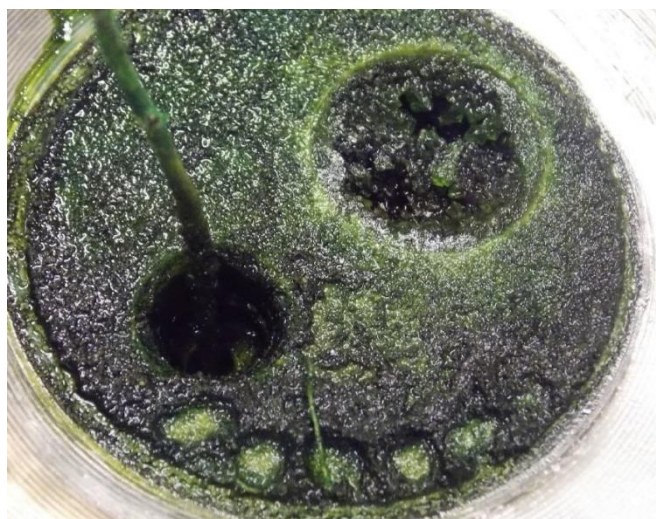
Figure 18 - green residue build-up on bottom flange following chronic HCl testing of Verdal
