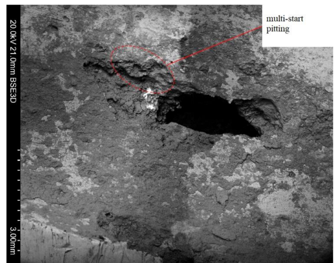
Figure 4 - Scanning Electron Micrograph of perforation (location of pipe failure)
