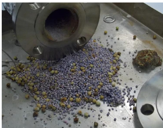
Figure 22 - following accelerated chronic testing, Loflosorb (purple balls) came out in good condition.
