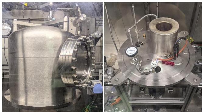
Figure 2: The "Bell Jar" suspended from its lifting arm (left) and the base plate (right), on which the Amersham heater jacket is mounted.
