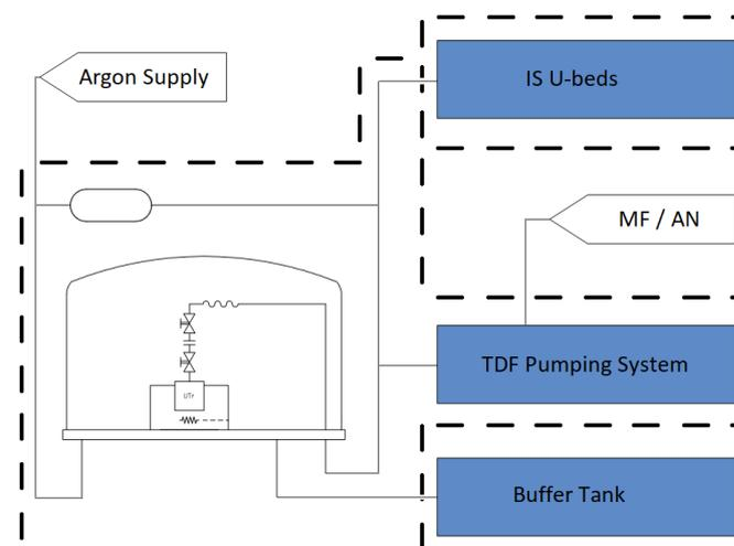
Figure 3: Simplified diagram of the Tritium Decanting Facility
