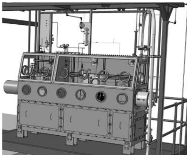
Figure 4: 3D render of the TDF glovebox, the bell is visible in the "closed" position in the main box
