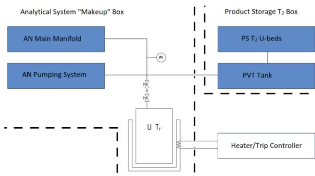
Figure 1: Simplified diagram of the AN "Makeup" Box decanting system
