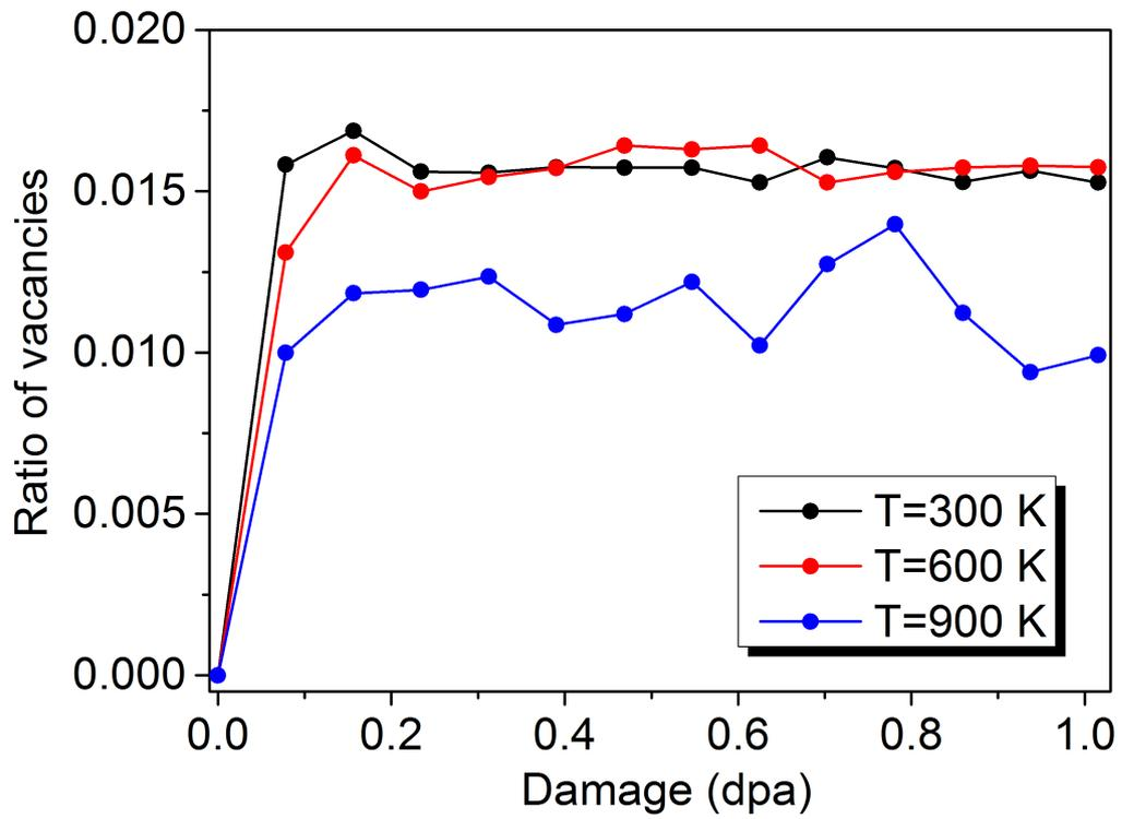
Figure 6. Ratio of single vacancies created in molybdenum as function of canonical damage introduced by Frenkel pair accumulation method at different temperatures.
