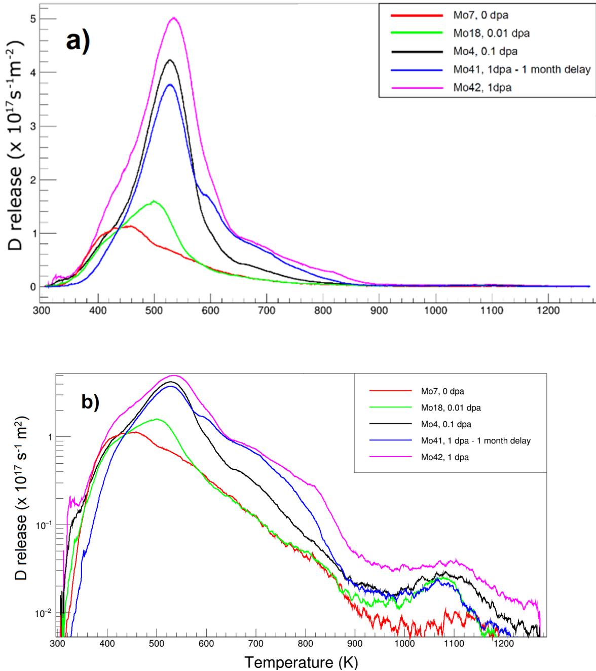
Figure 3. TDS spectra of deuterium in Mo samples with damage levels between 0 and 1 dpa. For samples Mo18, Mo4, and Mo42, spectra were taken 1 day after exposure to D plasma; for the sample Mo41, spectrum was taken 1 month after exposure. Linear plot (a); logarithmic plot (b).
