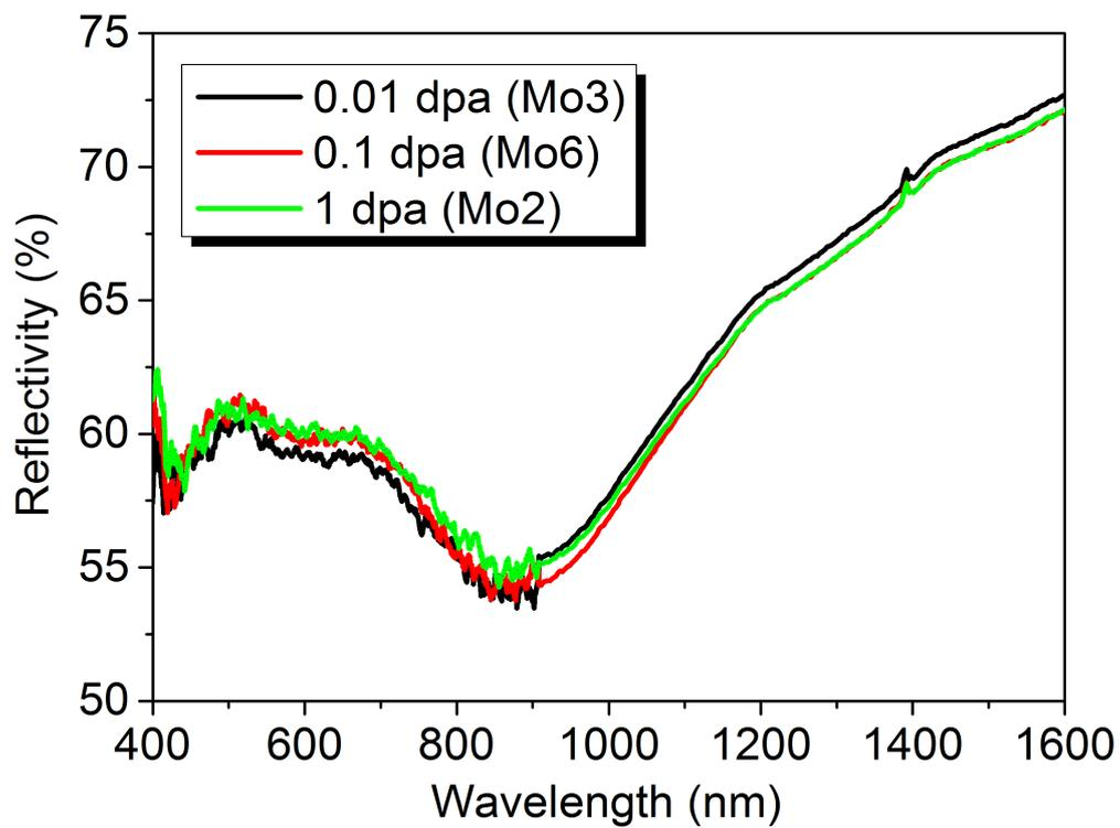
Figure 5. Total Mo reflectivity as a function of wavelength for samples irradiated to 0.01 dpa (Mo3), 0.1 dpa (Mo6), and 1 dpa (Mo2).
