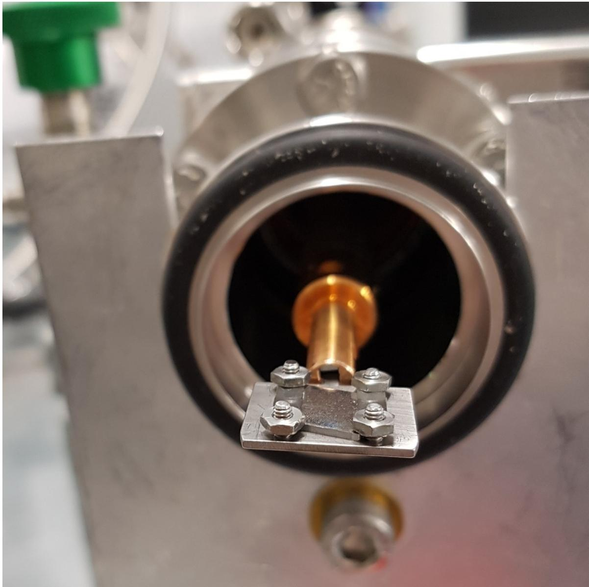
Figure 2. Molybdenum sample mounted to the sample holder.
