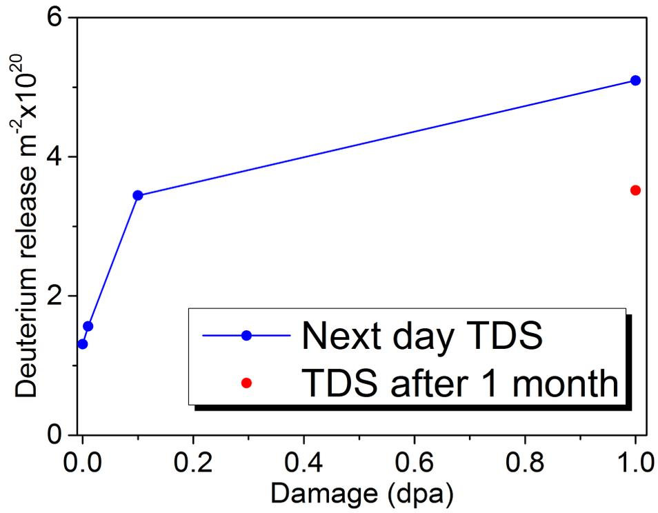
Figure 4. Overall deuterium inventory as function of canonical damage. For 1 dpa samples, results are shown for TDS performed next day (Mo42, blue point) and one month (Mo41, red point) after exposure.
