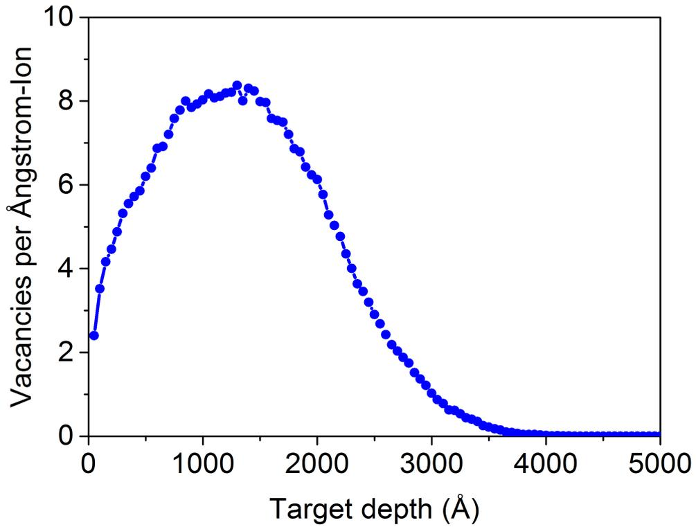
Figure 1. Number of vacancies created per incoming ion in 1 Å thick layer as function of depth as obtained using SRIM software for 1 MeV incoming Mo ions.
