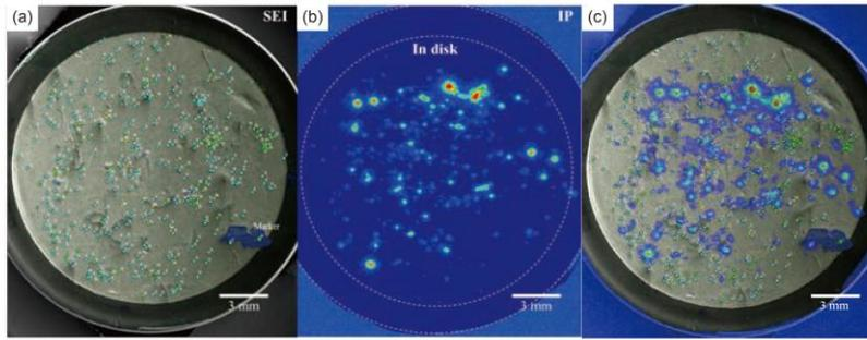
FIG. 9. EPMA image showing composition of dust particles (a). Small circles with superscript labels indicate the location and composition (C, O, Be and W) of dust particles. IP image showing tritium distribution on the indium disk (b) and superimposed image of (a) with (b) - (c).
