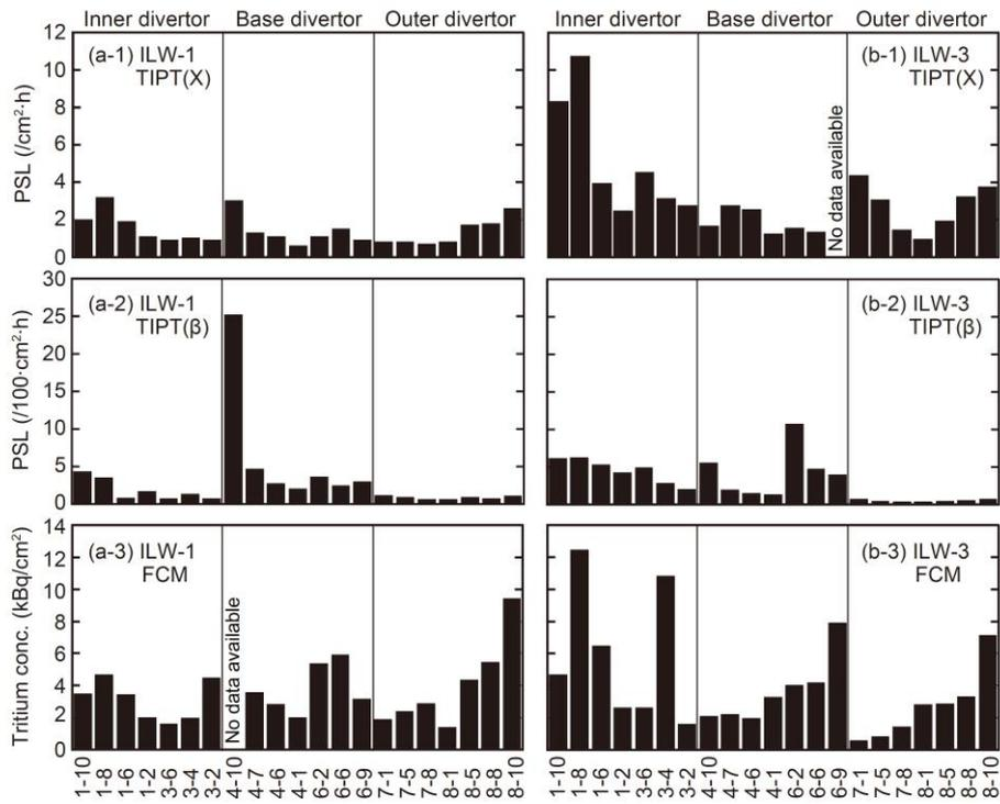
FIG.10. Tritium concentrations as measured by FCM and PSL intensities as measured by TIPT at ILW divertor tiles. No measurement available for ILW-3 sample 6-9 as measured by X-ray TIPT and ILW-1 sample 4-10 as measured by FCM.
