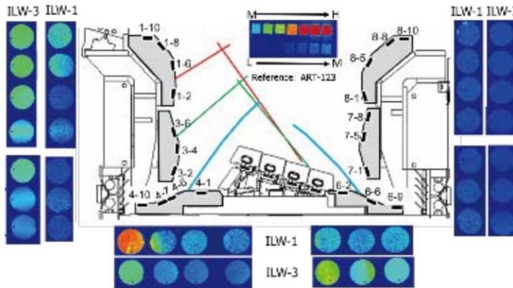
FIG.8. Imaging plate results of cored samples in ILW-1 and ILW-3, and tritium reference sample. Positions of cored samples are shown in a poloidal cross-section in which left-hand side is the torus inboard side. Coloured lines show the positions of the separatrix in three typical configurations, ILW-1 predominantly green, ILW-2 and 3 green and predominantly blue.
