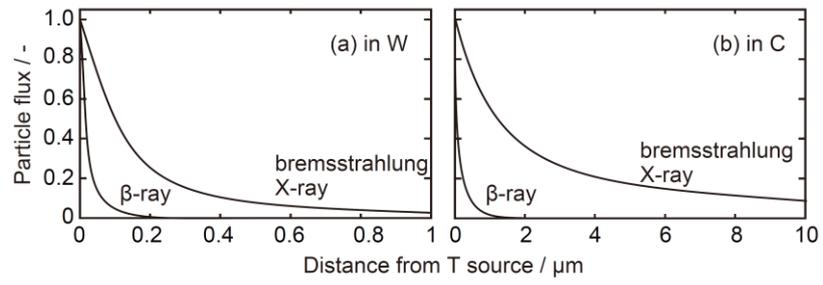
FIG.11. Intensity of particle flux dependent on transmission distance of  $\beta$ -rays and Bremsstrahlung X-rays for tritium in tungsten and carbon calculated by the Monte Carlo method. (a) in tungsten and (b) in Carbon.
