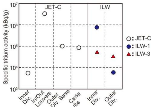
FIG.5. Specific tritium activities in dust particles after operated with JET-C, ILW-1 and ILW-3 as measured by FCM.
