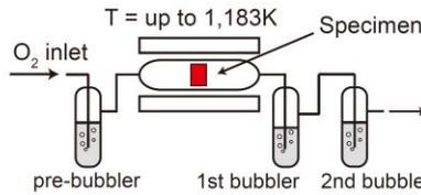
FIG. 3. Experimental set-up for tritium measurement using the full combustion method.
