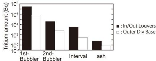
FIG.4. Quantitative measurement of tritium in dusts of In/Out Louvers and Outer Divertor Base at JET-C as measured by full combustion method.
