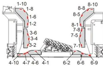
FIG.1. Cross-section of the JET-ILW divertor with marked position of specimen
