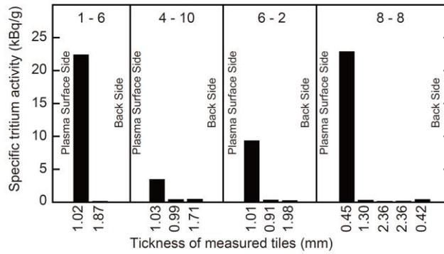
FIG.7. Depth profile of specific tritium activities in tiles after operated with ILW-3 as measured by FCM.
