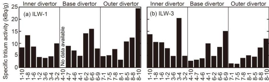
FIG.6. Specific tritium activities in tiles after operated with ILW-1 and ILW-3 as measured by FCM. No measurement available for ILW-1 sample 4-10.
