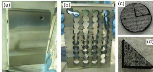
FIG.2. Photos of ILW-1 divertor Tile 4 and specimen for FCM: (a) divertor tile, (b) cored tile, (c) cored specimens and (d) cut-out specimen for tritium analysis by FCM.
