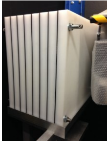
Figure 69 DIR shielding blocks.
