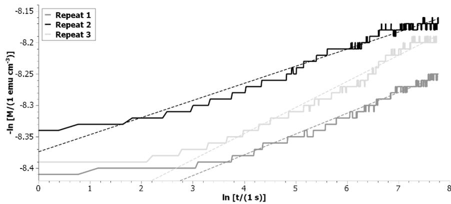
**Fig. 5** Natural logarithm of volume magnetisation versus natural logarithm of time for 3 repeat samples of the 7.5 % Zr tape at 20 K and 14 T - flux creep rates equal the line of best fit gradient (dashed lines)
