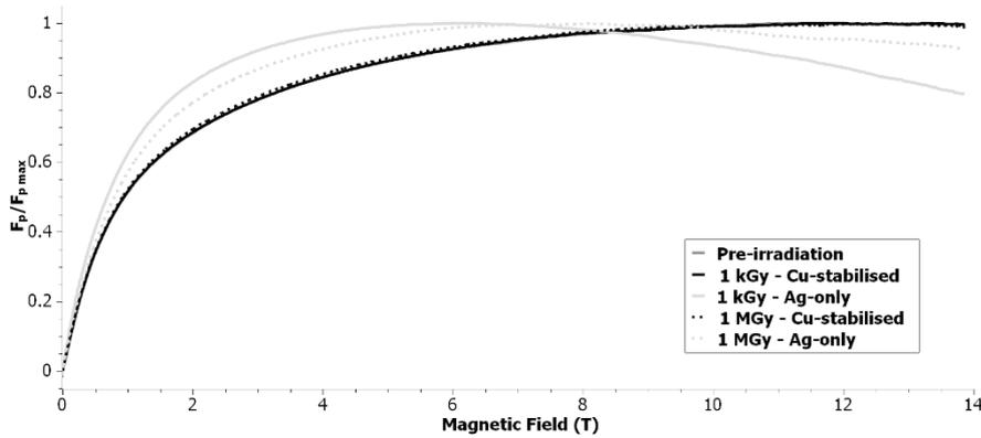
**Fig. 14** Normalised pinning force versus magnetic field strength for the 7.5 % Zr tape prior to gamma irradiation, and the Cu-stabilised and Ag-only samples after 1 kGy and 1 MGy gamma irradiation –  $F_p$  values calculated at 20 K
