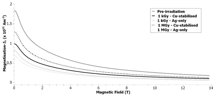
**Fig. 9** Magnetisation critical current density versus magnetic field strength for the 15 % Zr tape prior to gamma irradiation, and the Cu-stabilised and Ag-only samples after 1 kGy and 1 MGy gamma irradiation –  $J_c$  values calculated at 20 K
