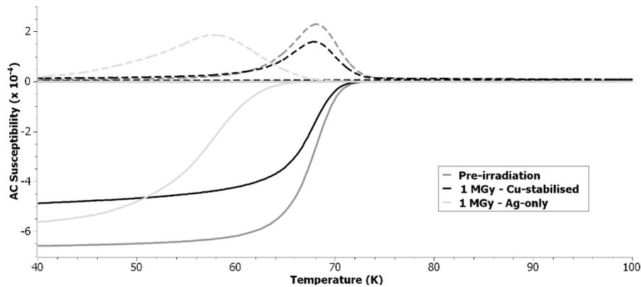
**Fig. 21** AC susceptibility versus temperature for the 15 % Zr tape prior to gamma irradiation, and the Cu-stabilised and Ag-only samples after 1 MGy gamma irradiation – susceptibility values at 14 T
