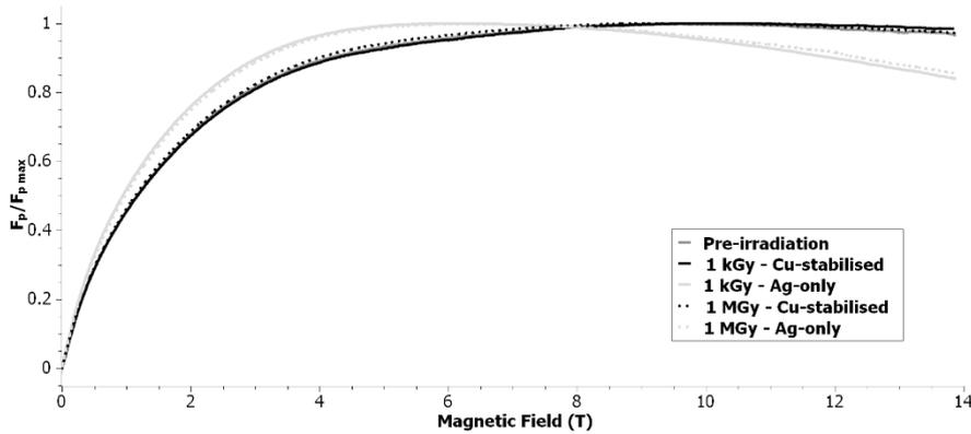
**Fig. 15** Normalised pinning force versus magnetic field strength for the 15 % Zr tape prior to gamma irradiation, and the Cu-stabilised and Ag-only samples after 1 kGy and 1 MGy gamma irradiation –  $F_p$  values calculated at 20 K
