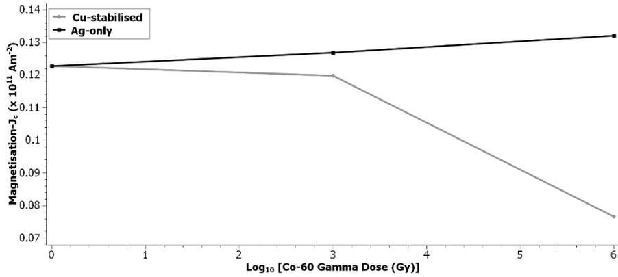
**Fig. 10** Magnetisation critical current density values at 20 K and 13.85 T for the 0 % Zr tape prior to gamma irradiation, and the Cu-stabilised and Ag-only samples after 1 kGy and 1 MGy gamma irradiation
