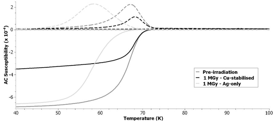
**Fig. 20** AC susceptibility versus temperature for the 7.5 % Zr tape prior to gamma irradiation, and the Cu-stabilised and Ag-only samples after 1 MGy gamma irradiation – susceptibility values at 14 T
