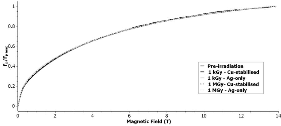
**Fig. 13** Normalised pinning force versus magnetic field strength for the 0 % Zr tape prior to gamma irradiation, and the Cu-stabilised and Ag-only samples after 1 kGy and 1 MGy gamma irradiation –  $F_p$  values calculated at 20 K
