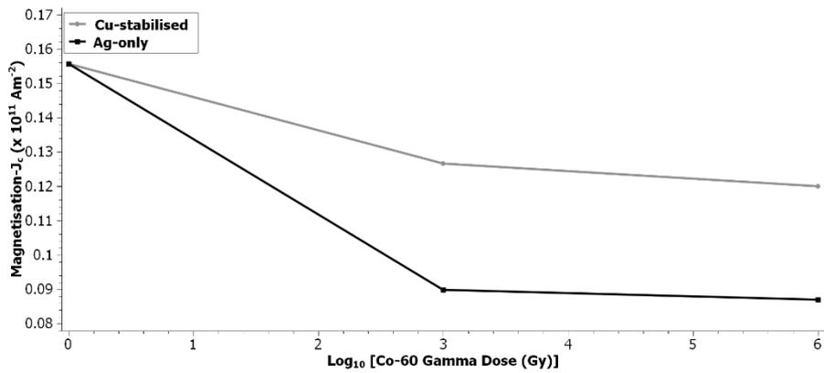
**Fig. 11** Magnetisation critical current density values at 20 K and 13.85 T for the 7.5 % Zr tape prior to gamma irradiation, and the Cu-stabilised and Ag-only samples after 1 kGy and 1 MGy gamma irradiation
