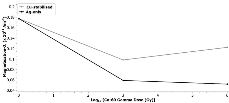
**Fig. 12** Magnetisation critical current density values at 20 K and 13.85 T for the 15 % Zr tape prior to gamma irradiation, and the Cu-stabilised and Ag-only samples after 1 kGy and 1 MGy gamma irradiation
