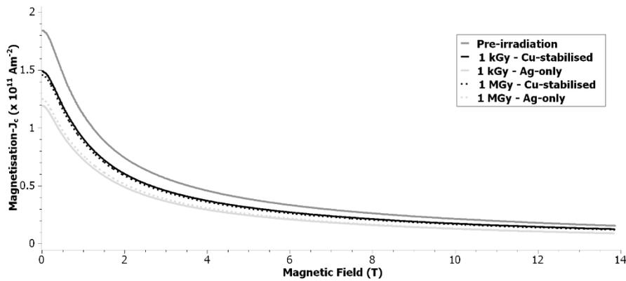
**Fig. 8** Magnetisation critical current density versus magnetic field strength for the 7.5 % Zr tape prior to gamma irradiation, and the Cu-stabilised and Ag-only samples after 1 kGy and 1 MGy gamma irradiation –  $J_c$  values calculated at 20 K
