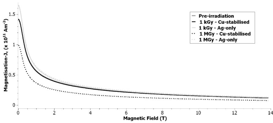
**Fig. 7** Magnetisation critical current density versus magnetic field strength for the 0 % Zr tape prior to gamma irradiation, and the Cu-stabilised and Ag-only samples after 1 kGy and 1 MGy gamma irradiation –  $J_c$  values calculated at 20 K
