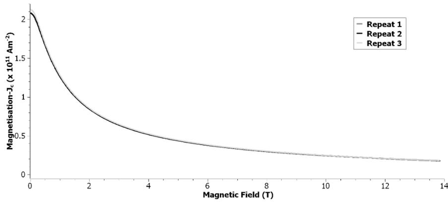
**Fig. 2** Magnetisation critical current density versus magnetic field strength for 3 repeat samples of the 7.5 % Zr tape –  $J_c$  values calculated at 20 K
