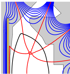
Figure 3. Contours of flux (blue/red) due to central solenoid (yellow), plus the four odd SHs which give \mathbf{B}_p = \nabla B_p = \mathbf{0} at the red circle. The boundary of shot 45272 at 750ms is in black.
