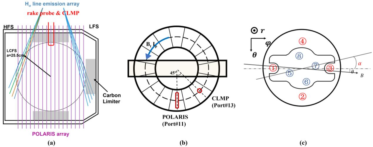
**Figure 1.** Arrangement of the main diagnosis. (a) Cross-section of J-TEXT tokamak, viewing lines of the J-TEXT PDA (in blue color) and POLARIS (in magenta color), respectively. The CLMP locates at  $r = 23.5\text{cm}$  and the rake probe array was used for measuring floating potential at  $r - a = -3 \sim 2\text{ cm}$ . (b) Top view of J-TEXT tokamak, POLARIS and CLMP are toroidally separated by  $45^\circ$ . (c) The configuration of CLMP array.
