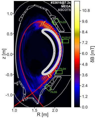
**Figure 1.** Poloidal cross section of AUG showing a MEGA calculation of the magnetic field perturbation associated with an ELM (colour bar). A fast-ion orbit calculated with ASCOT is in light grey, FILD probes are marked in green and the red curve shows the confined plasma separatrix.
