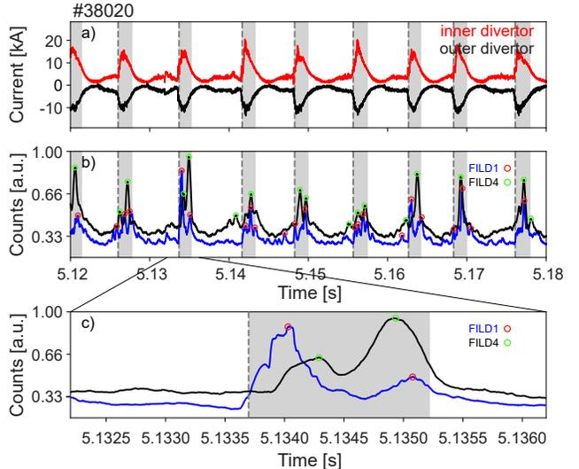
**Figure 2.** (a) Time trace of the inner and outer divertor current. (b) Time trace of FILD1 and FILD4. The most prominent spikes in the signal are circled. (c) Close-up of FILD1 and FILD4. The times of ELM onset, as measured by the initial rise in the divertor current, are marked by the dashed grey lines and the ELM durations are shaded.
