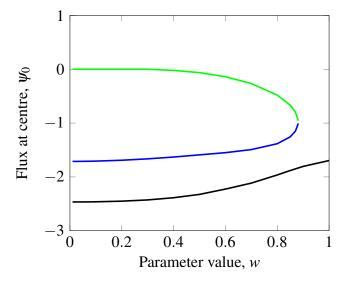
**Figure 4.** Bifurcation diagram for our toy model varying the parameter w with C = 2.9 and  $\psi_p = -1.0$ . The most negative solution is always there but at  $w \approx 0.88$  two new solutions appear at a fold bifurcation and persist as w decreases.
