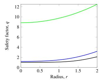
**Figure 13.** Plot of the safety factor profiles for the three solutions of the large aspect ratio GSE with C = 2.9.
