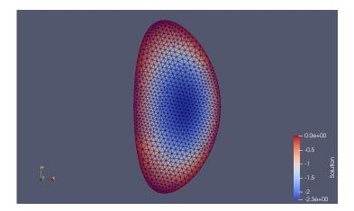
**Figure 9.** Example of solution mesh, generated with Gmsh, and solution, computed by Firedrake/Defcon, for a plasma with elongation  $\kappa = 2$ , triangularity  $\delta = 0.3$ , and major radius  $R_0 = 3$ .
