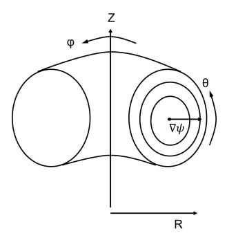
**Figure 1.** Cartoon of the coordinate system used for the Grad–Shafranov equation.
