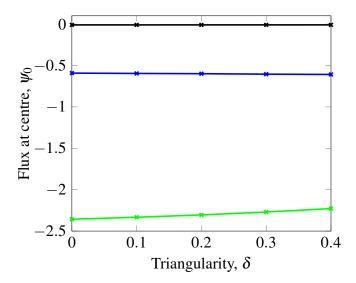
**Figure 11.** Scan of plasma triangularity major radius  $R_0$  with fixed minor radius a = 1 with circular cross section which amounts to a scan in aspect ratio of the torus. The central value of poloidal magnetic flux  $(\psi_0)$  for the three solutions is shown.
