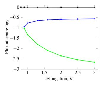
**Figure 10.** Scan of plasma elongation,  $\kappa$ , with fixed major radius  $R_0 = 3$  with fixed minor radius a = 1. The central value of poloidal magnetic flux  $(\psi_0)$  for the three solutions is shown. Two solution branches coalesce at around  $\kappa = 0.9$  and only the trivial solution exists for smaller values of elongation.
