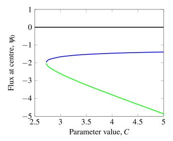
**Figure 3.** Bifurcation diagram for our toy model varying the parameter C with w = 0.05 and  $\psi_p = -1$ . The trivial solution always exists but at  $C \approx 2.7$  two new solutions appear at a fold bifurcation and persist as C increases.
