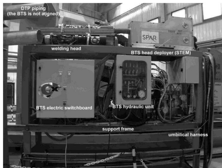
Figure 5 Overview of the 160 mm piping BTS on divertor test platform (DTP) [97]
