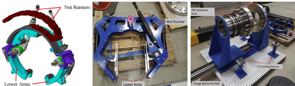
Figure 22 Prototype flange bolting tool (FBT) and mock-up test rig for DN300 pipe [103]
