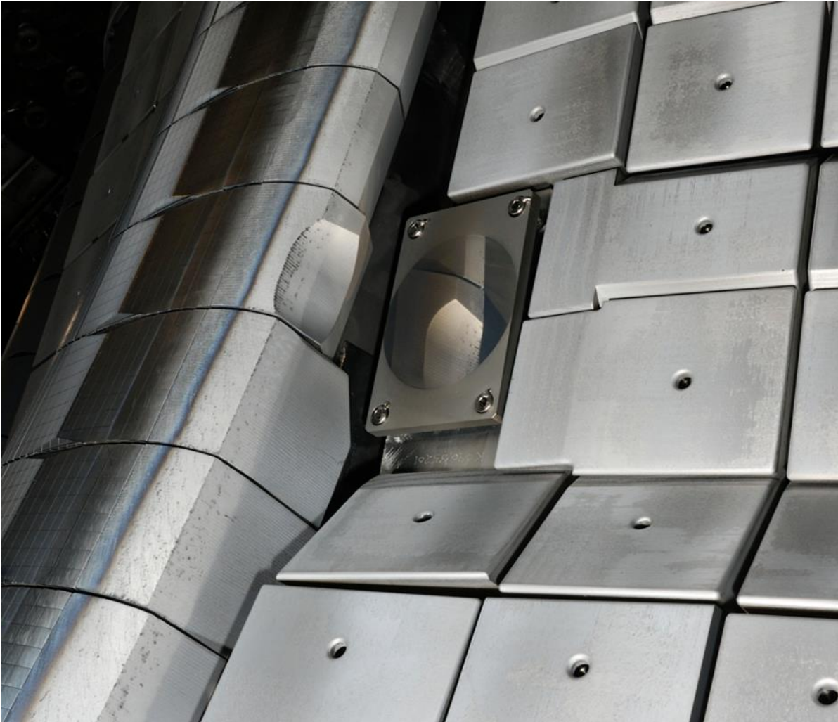
Figure 15 In-vessel mirror for JET FIR diagnostic (installed in 1992, photographed in 2014 during in-vessel photographic survey)
