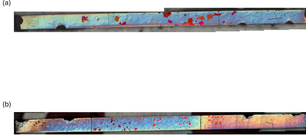
Fig. B. 1. Chosen 001 oriented grains from EBSD analysis of (a) Fe 3 Cr, and (b) Fe 5 Cr represented in red colour. Figure width is 25 mm.
