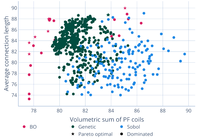
FIG. 9: Feasible solutions in the objective space for experiments I (red), V (blue), and VII (green) in Table IV. Pareto optimal solutions are denoted with a star and dominated solutions with a circle.
