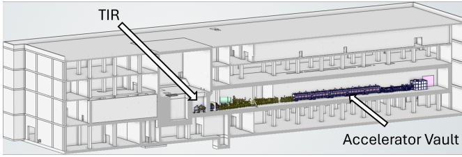
Figure 3: CAD model of the building housing the accelerator. Labeled is the accelerator vault and the Target Interface Room (TIR). A slice has been taken in the Y-plane
