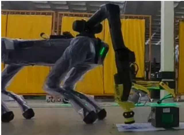
FIGURE 1: Sample retrieval trial using a robotic mobile manipulator equipped with a swabbing tool for radiological contamination monitoring (Source: Robotics & AI Collaboration/UKAEA)
