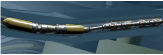
Fig. 2 Welding tool and in-bore deployment system
