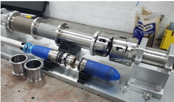
Fig. 5 Weld tool and welded P91 and 316L samples
