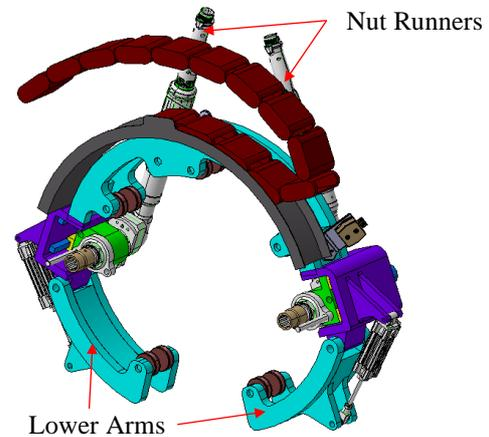
Fig. 3 Flange Bolting Tool (FBT) concept
