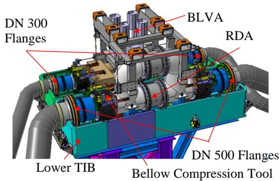
Fig. 2 Flanges and pressure relief assemblies
