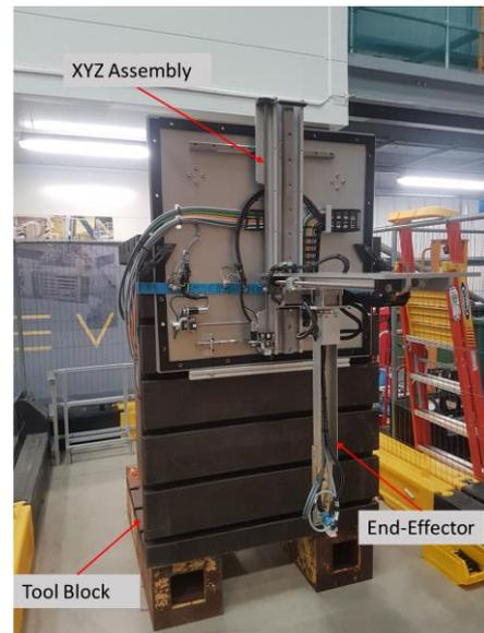
Fig. 8 XYZ test rig at the RACE facility, Culham
