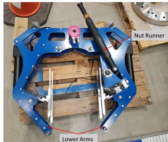
Fig. 6 Prototype FBT at the RACE facility, Culham
