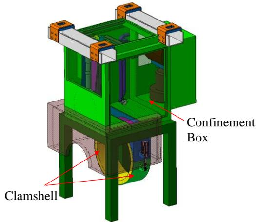
Fig. 4 Confinement Tool (CT) concept
