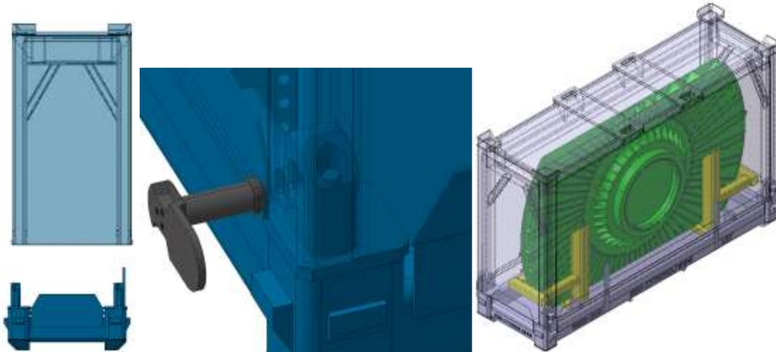
Fig. 21 Lid of the Waste Storage Basket above the base frame (left), locking pins (centre), and the full Waste Storage Basket assembly (right).
