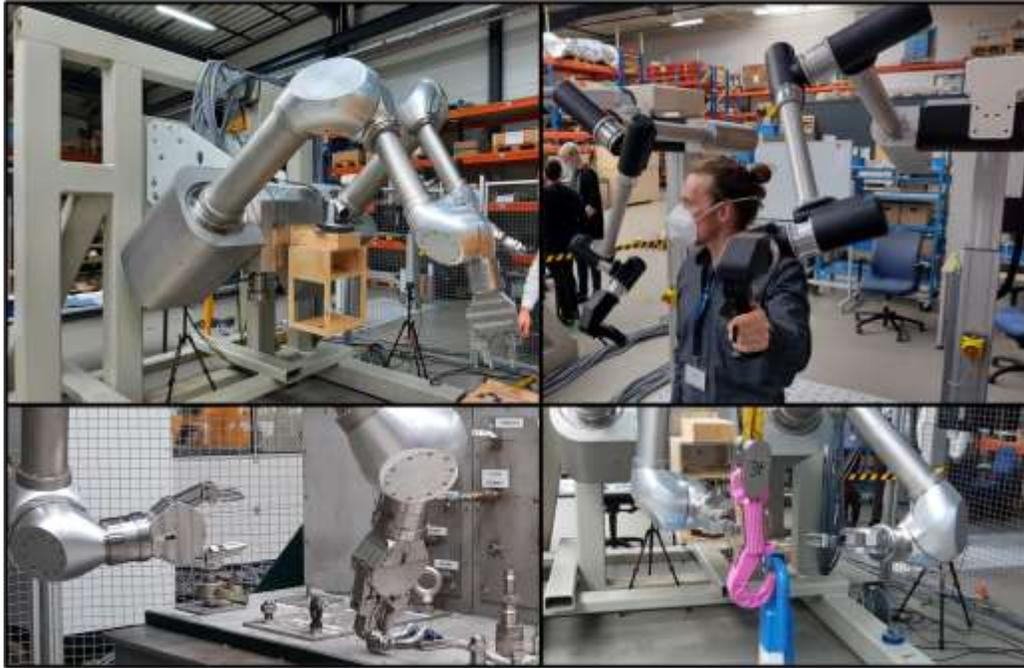
Fig. 9 Images from Factory Acceptance Testing of the Telbot Manipulators
