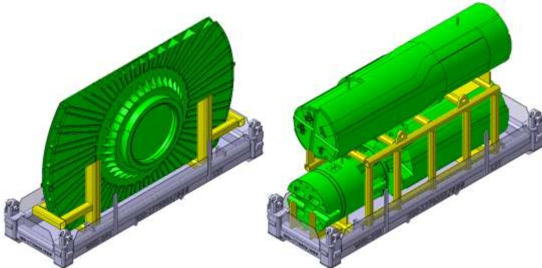
Fig. 20 Waste Storage Basket base frame and example component support frames for the parts of the target wheel (left) and moderator reflector plug shaft (right).
