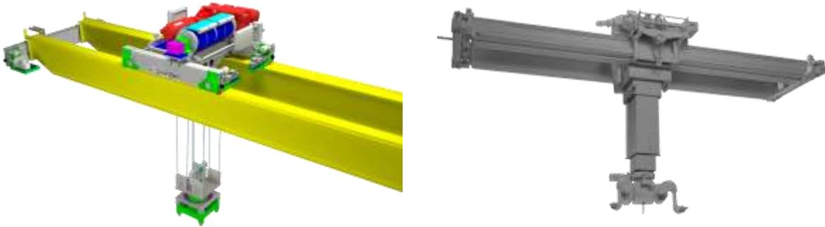
Fig. 7 Design images of the Grapple Crane (left) and Manipulator Crane (right)
