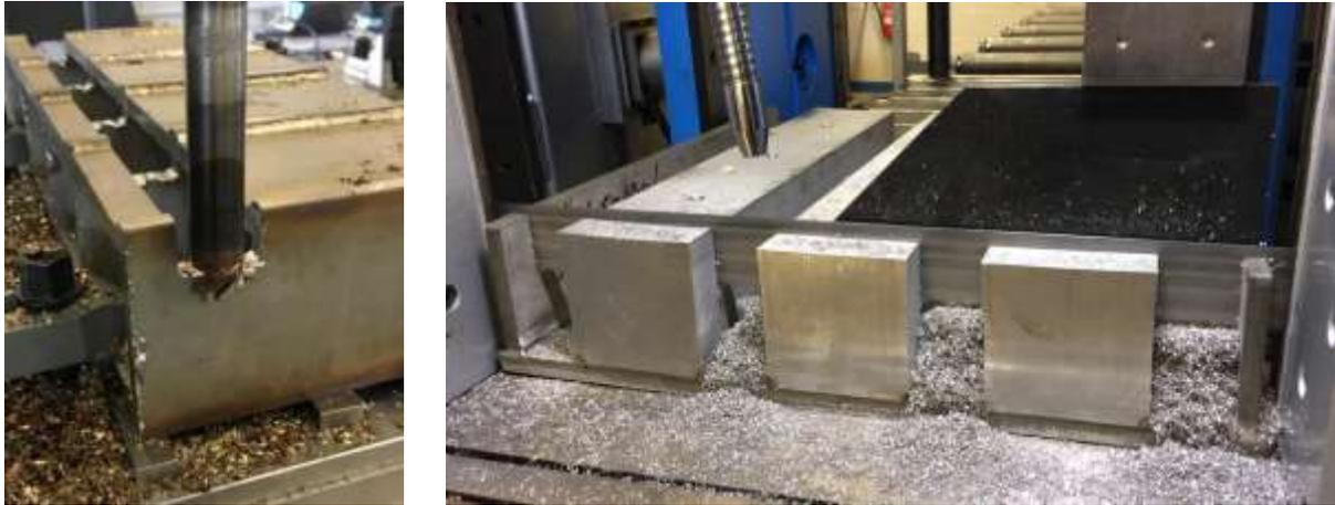
Fig. 11 Cutting feasibility trials carried out by UKAEA
