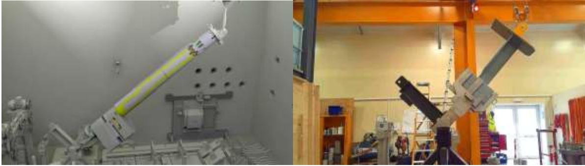
Fig. 13 VR simulation of laying over the Moderator Reflector Plug (left) compared to Factory Acceptance Testing of the layover cup (right)
