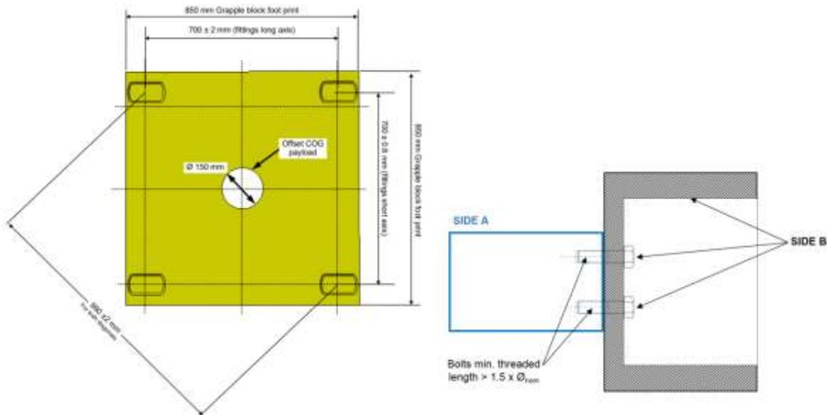
Fig. 6 The 25 tonne grapple interface (left) and the gripper interface (right)
