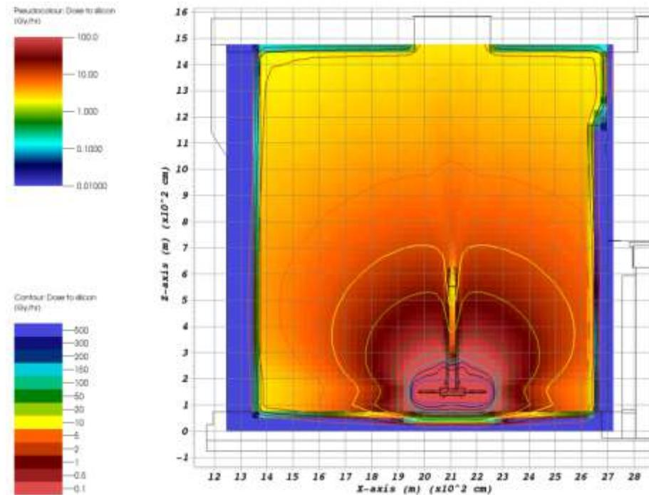
Fig. 4 Gamma dose to silicon near to the ESS Target Wheel after 5 years of irradiation.
