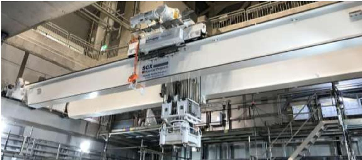
Fig. 8 The Grapple Crane installed in the Active Cells
