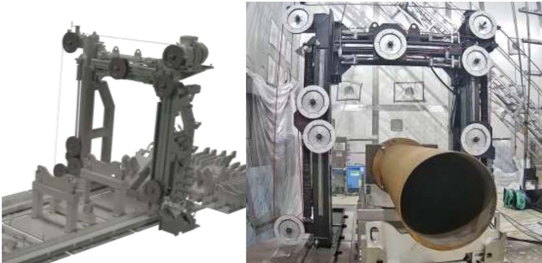
Fig. 14 The Shaft Cutting Station saw design (left) and during cutting trials (right)
