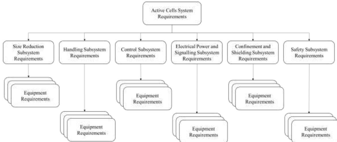
Fig. 3 Requirement breakdown structure for the Active Cells System
