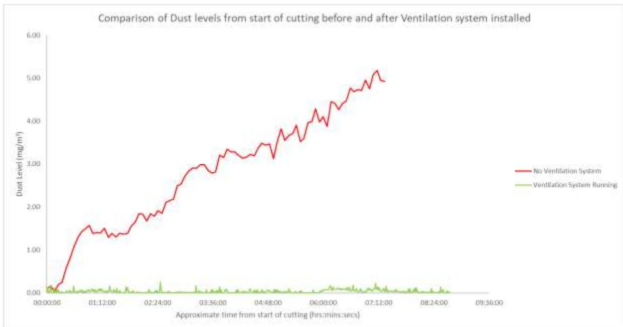
Fig. 16 Dust measurements close to the cut location during site cutting trials with and without a ventilation system in operation.
