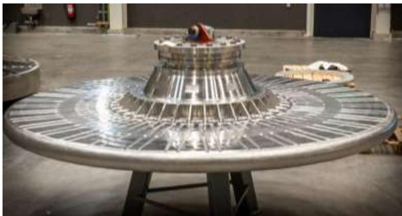
Fig. 1 The ESS Target Wheel © ESS
