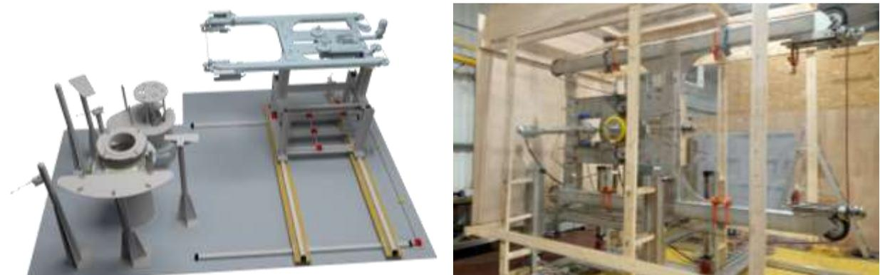
Fig. 17 The Machining Station design (left) and during cutting trials (right)
