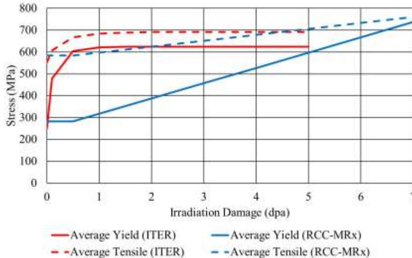
Fig. 10 Effect of neutron irradiation damage on the yield and tensile strength of 316L Stainless Steel.
