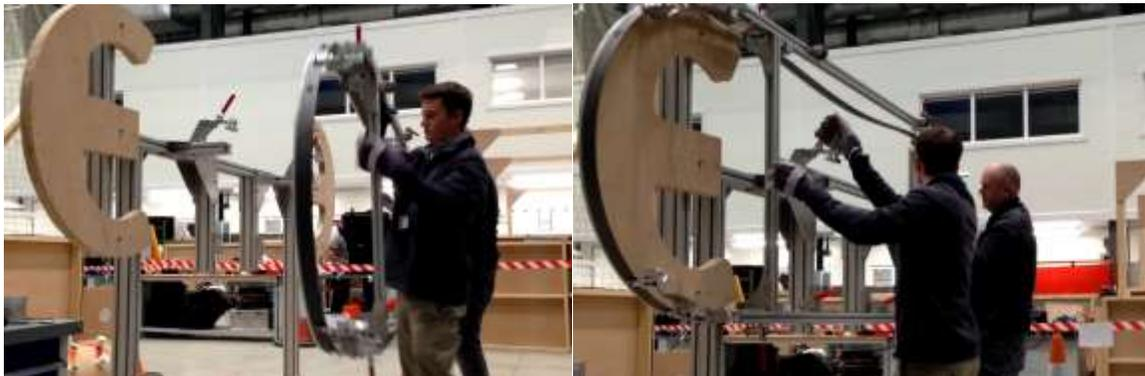
Fig. 12 Feasibility trials for remote-handling compatible change of a bandsaw blade.
