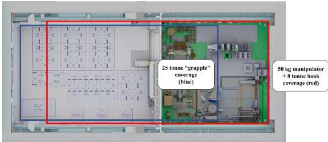
Fig. 5 Plan view of the Active Cells showing deployment areas for the 25 tonne and 50 kg handling capabilities.
