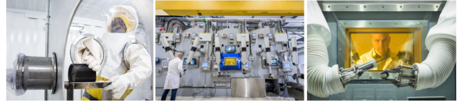
Fig. 6. Gloveboxes where the operator is wearing special gloves for protection while analysing/examining hazardous material or using 'master-slave' robotic manipulator system for the enhanced safety measures. Sources: U.S. Department of Energy and UKAEA.
