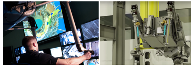
Fig. 9. Mascot is two-armed bilateral teleoperation system allowing remote maintenance and reconfiguration of the JET tokamak. Source: UKAEA.
