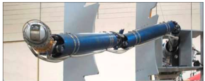
Fig.6. WEST AIA in mock-up test.
