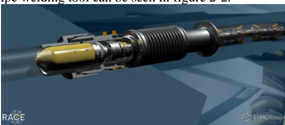
Figure 2-2: DEMO in-bore laser welding tool
