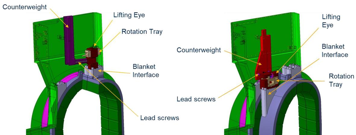
Figure 10 – Crane-lifted counterbalance concepts
