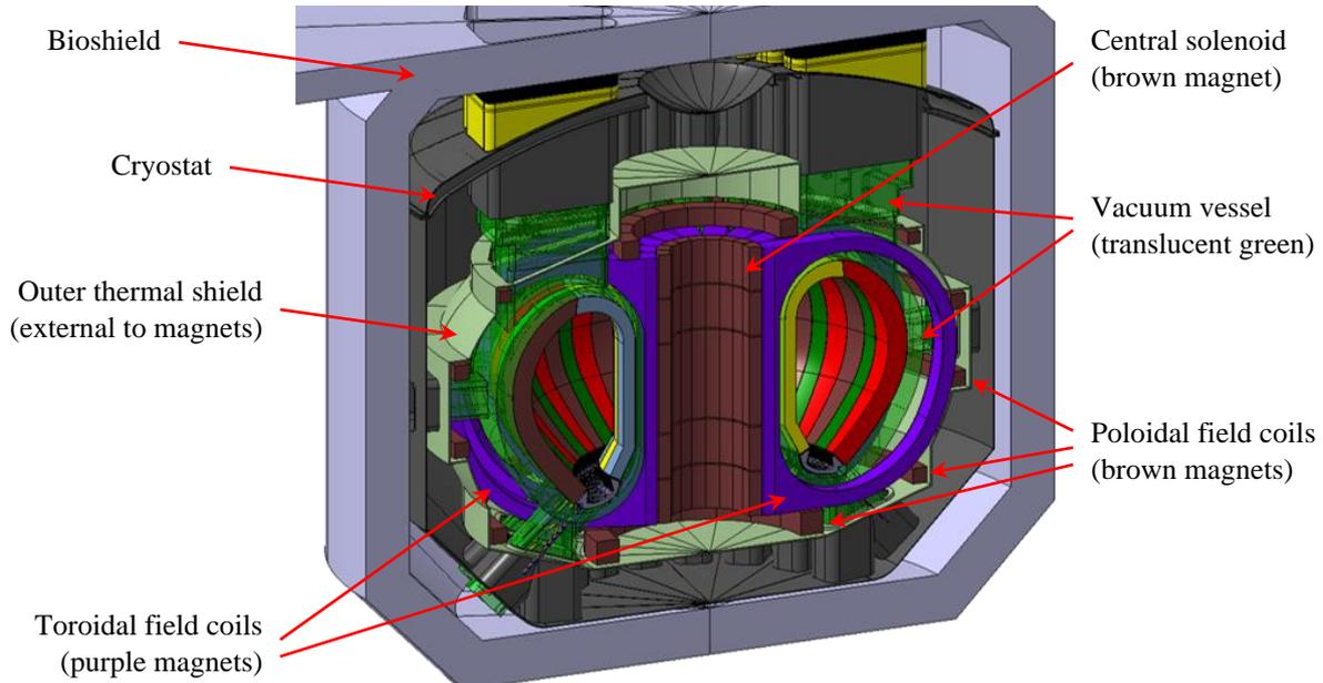
Figure 4 – Cross-section of DEMO within the bioshield.
