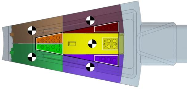
*Figure 7 – Plan view on one sector (22.5°) of the vessel (grey), showing 5 blanket segments (coloured) together with their pipe connections and centres of mass relative to the port.*
