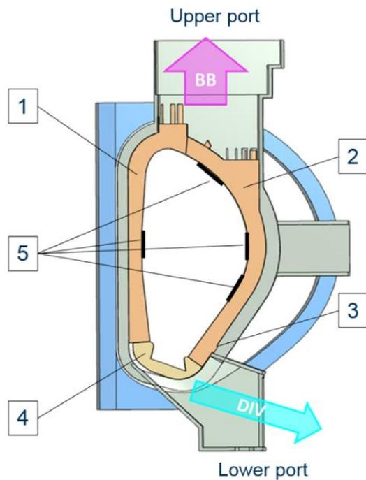
1. Inboard Breeding Blanket (IBB): Segmented components that line the inner wall of the vacuum vessel. 2 per vessel sector. Require replacement several times during the life of DEMO. Length 12m. Mass up to 60 tonnes.
