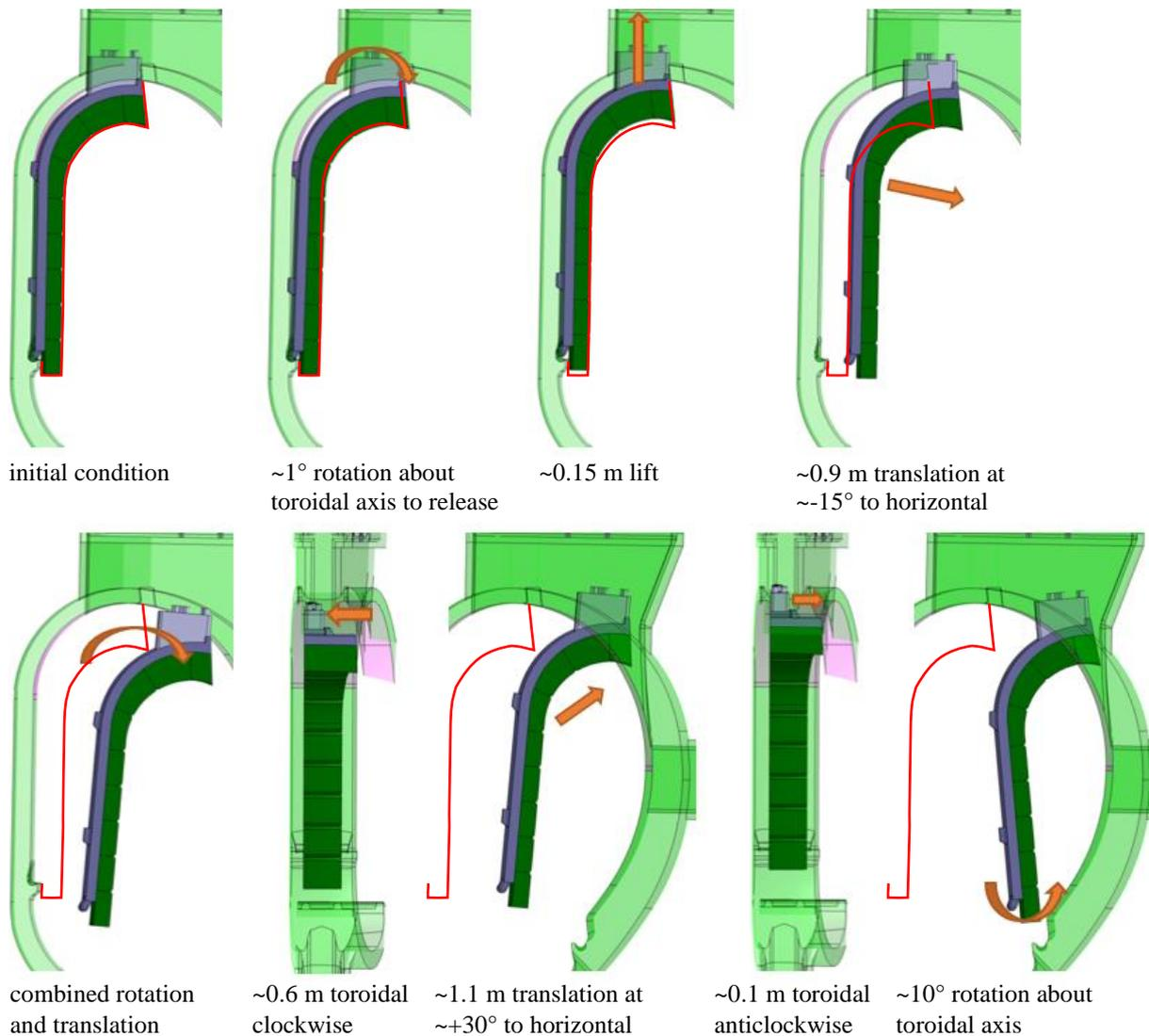
Figure 8 – Typical sequence of operations for Inner Breeding Blanket (IBB) removal, with adjacent blanket indicated in red outline
