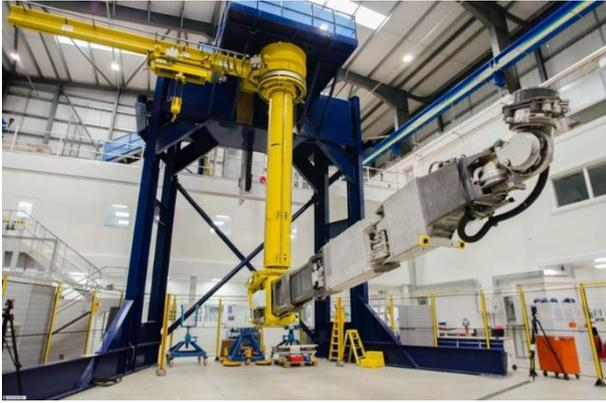
Figure 28 – Refurbished TARM installed on a bespoke remote maintenance testing stillage at UKAEA.
