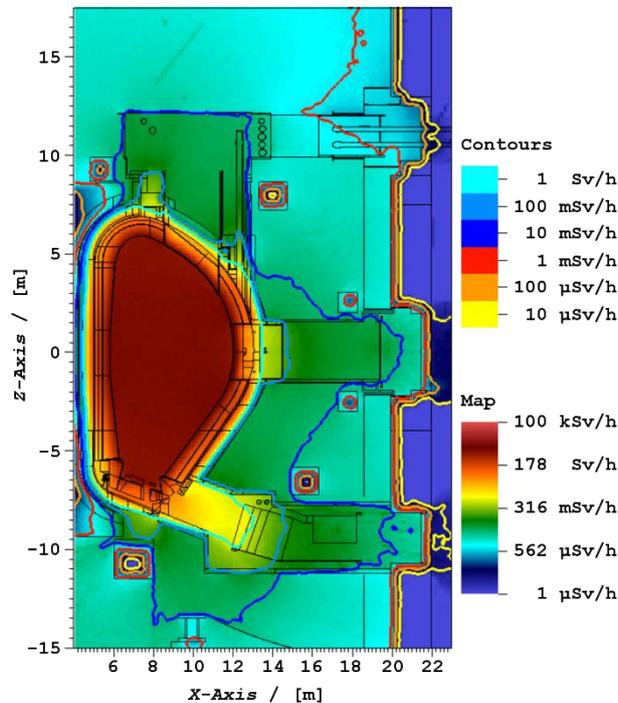
Figure 3 – Estimated dose rate in DEMO in a vertical plane through the port centre at the start of maintenance, approximately 1 month after deuterium-tritium plasma operations.
