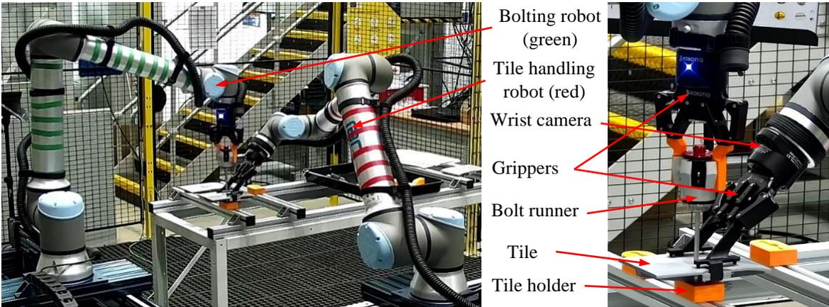
Figure 30 – Automated tile replacement
