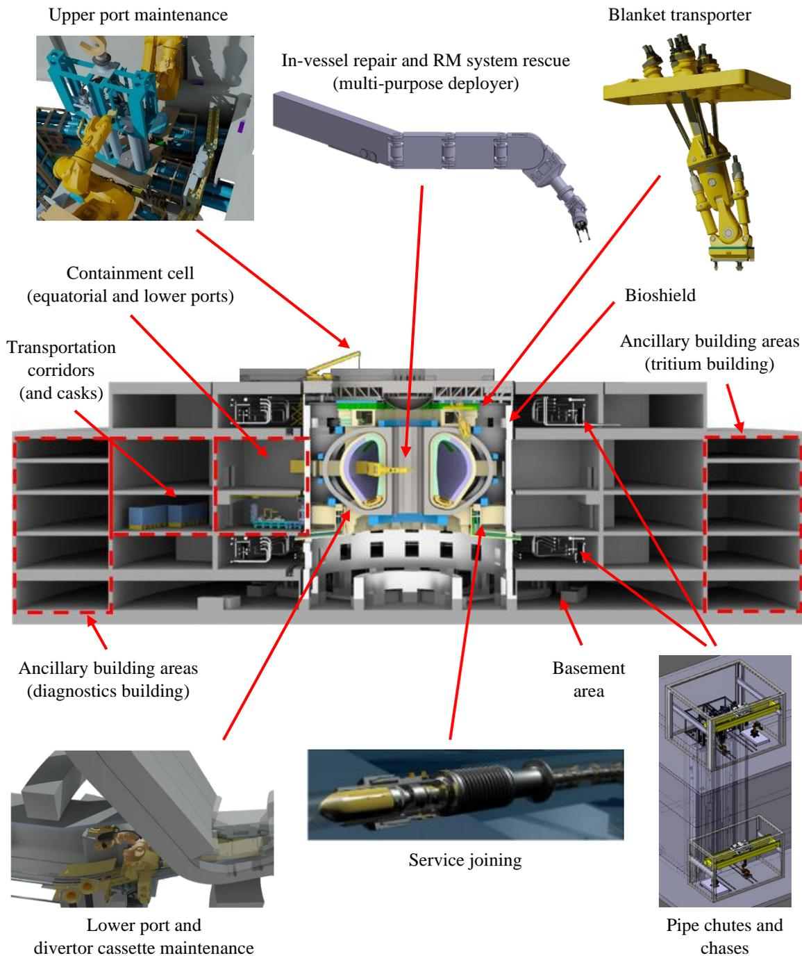
Figure 16 – Cross-section of DEMO reactor building concept accounting for remote maintenance space requirements (upper maintenance hall omitted for clarity)
