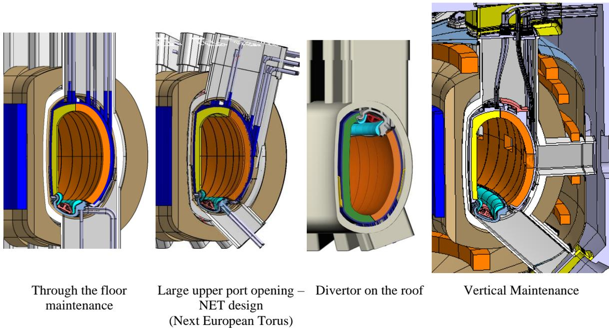
Figure 2 – DEMO port configurations considered for down-selection in 2013
