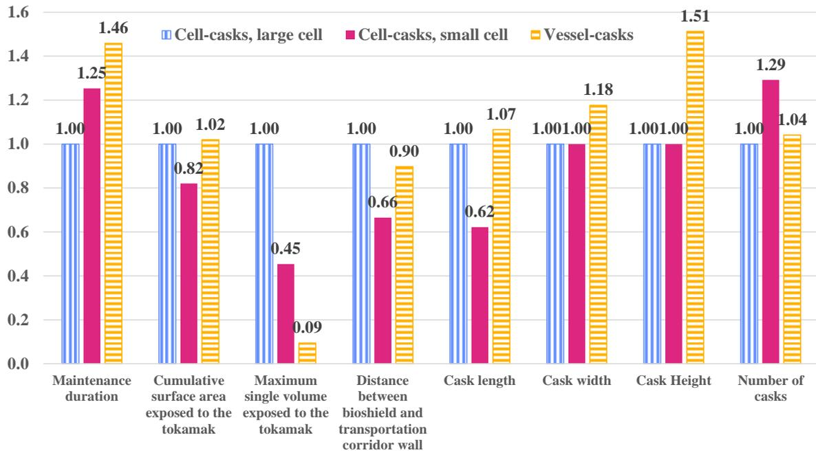
Figure 20 – Comparison of metrics for the large cell, small cell and the vessel cask approaches for the maintenance of the Lower Port.
