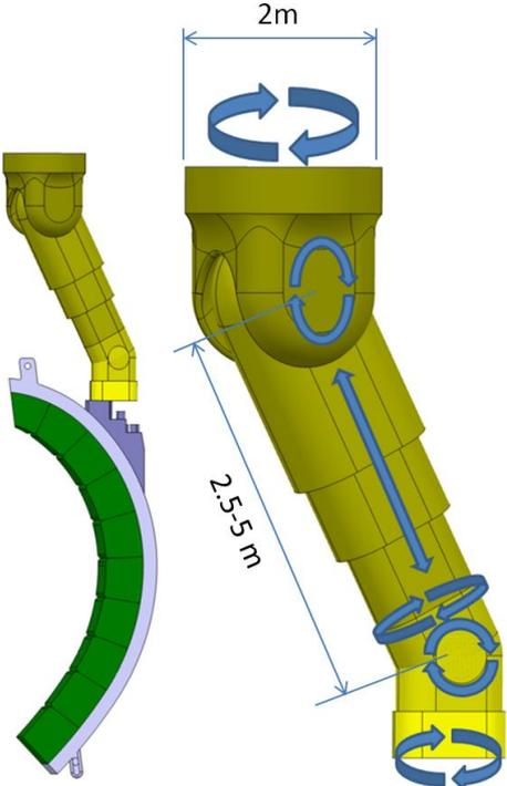
Figure 11 – Crane-lifted in-line manipulator concept.
