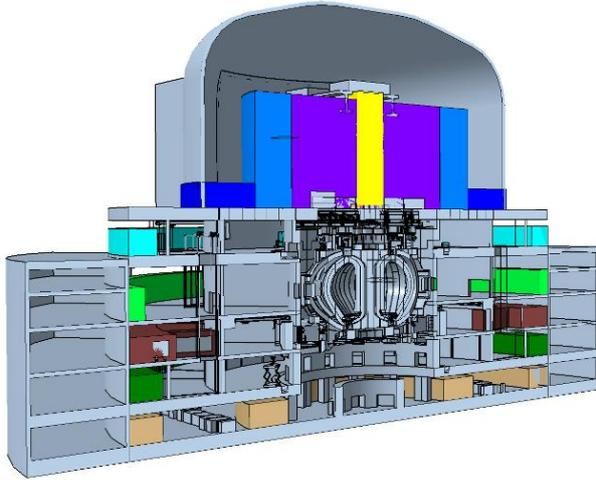
Figure 17 – DEMO space requirement analysis: maintenance volumes are shown as coloured blocks
