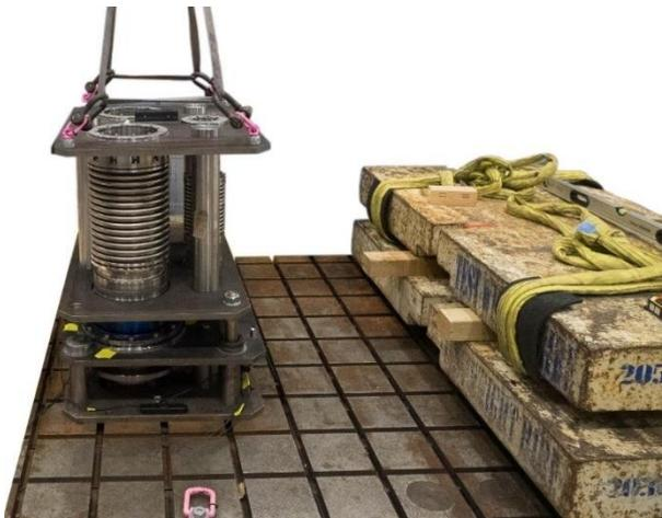
Figure 27 – Passive alignment mechanism testing showing pipe module dead-weight simulant at right
