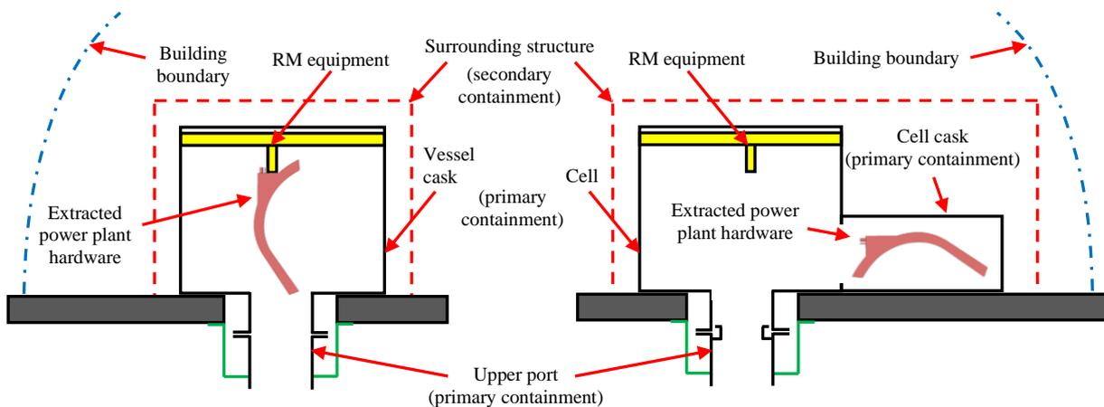
Figure 18 – Illustration of alternative confinement approaches: vessel cask (left), cell cask (right)
