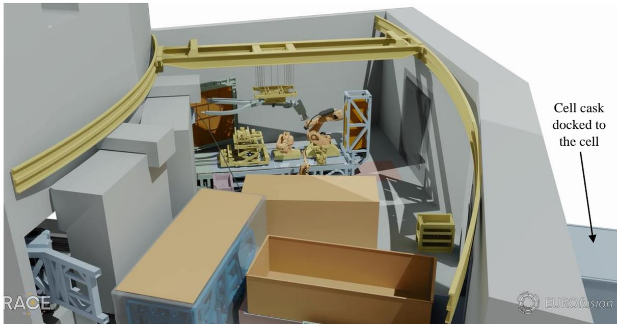
*Figure 19 – Image of the large port cell approach for maintenance of the lower port*
