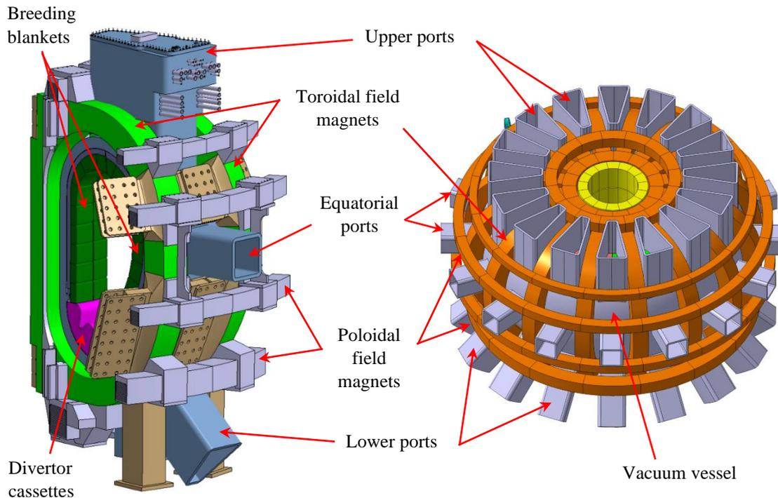
Figure 1 – Left: section view of one machine sector; right: the magnetic cage, vessel, and ports
