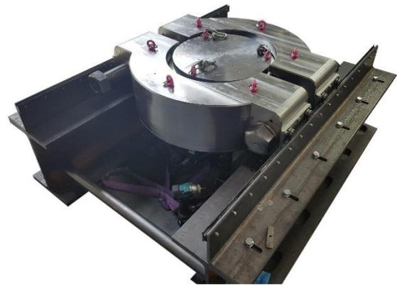
Figure 26 – Mechanical Pipe Connector proof-of-principle test bench isometric views
