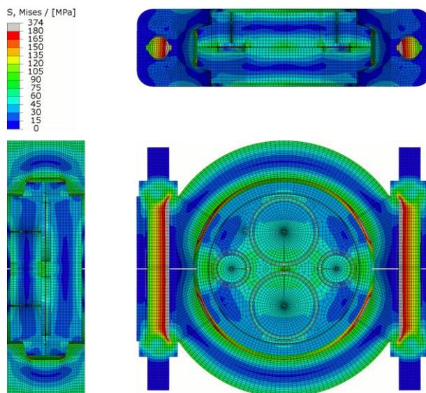
Figure 25 – Finite Element study of MPC concept design 2. Mid-plane equivalent stress distributions at 550 °C and 96 bar (third angle view).
