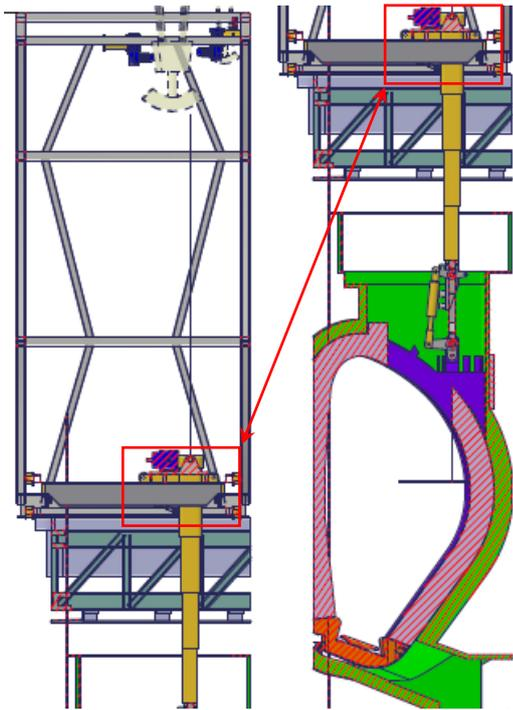
Figure 12 – End-effector mounted on a telescopic mast.
