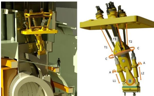
Figure 13 – Left: concept of HKM blanket mover operation (crane lift of HKM attached to Outboard Breeding Blanket segment); right: Detail of the six degrees-of-freedom of the HKM
