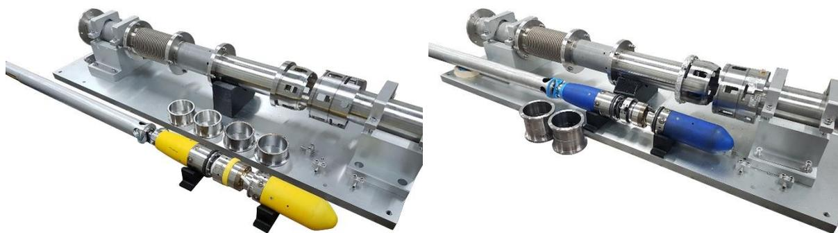
Figure 22 – Laser cutting tool (left) and welding tool (right) both with samples in P91 and 316L
