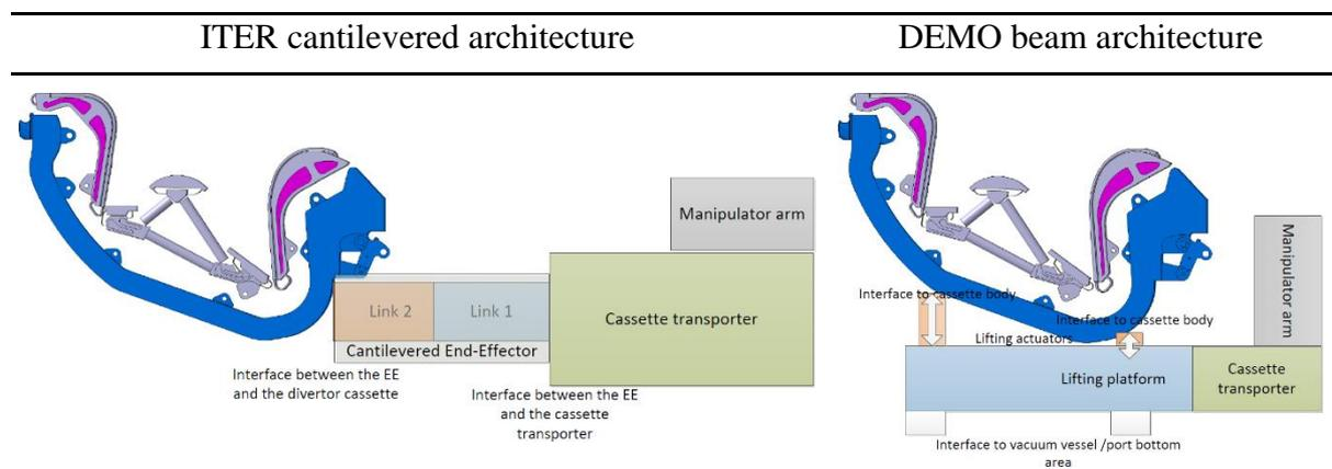
Figure 14 – Divertor transporter architecture comparison
