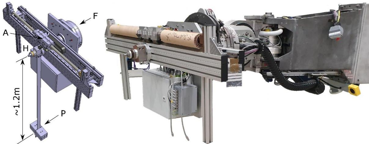
Figure 29 – Left: flexible pendulum model used to validate APCS; right: partial installation of flexible pendulum on TARM
