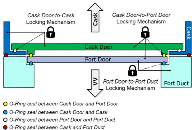
Figure 21 – Contamination Control Door (CCD) concept applied to a vessel cask
