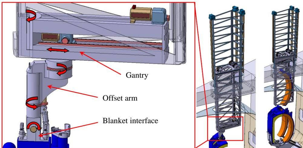
Figure 9 – Gantry crane with end-effector on a telescopic frame.
