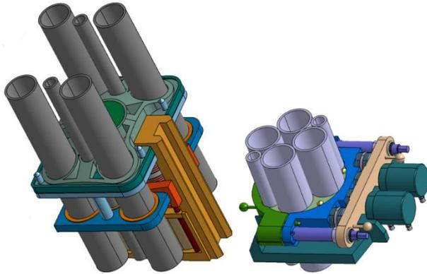
Figure 24 – Mechanical Pipe Connector designs: concept design 1 (left), concept design 2 (right).
