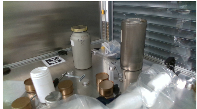
Figure 1: The glovebox mock-up and the manipulation system with representative cylindrical containers to store radioactive substances.
