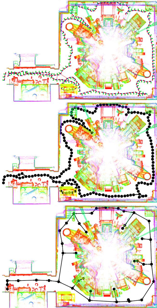
FIGURE 14. Building a topological map from the SLAM pose graph at JET. Top: SLAM pose graph, red edges indicate loop closures. Middle: Automatically constructed topological map. Bottom: Final topological map after manual pruning and adjustment for mission objectives.
