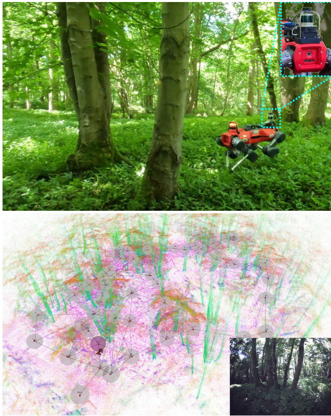
FIGURE 18. ANYmal Monitoring in Wytham Woods. Top: ANYmal navigating the forest. Bottom: Topological map and pointcloud used by the robot to navigate in a 50\text{ m} \times 35\text{ m} forest patch, with robot's front camera view overlaid.
