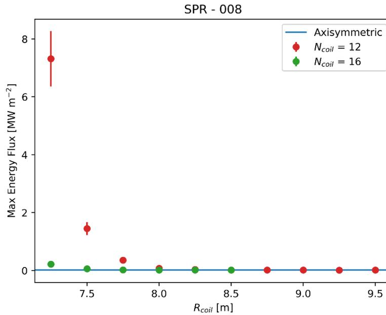
**Fig. 2.** Dependence on  $R_{\text{coil}}$  and  $N$  of maximum power flux due to lost  $\alpha$ -particles in STEP design with  $R_0 = 3.6\text{m}$ ,  $B_0 = 2.3\text{T}$ ,  $I_p = 23.2\text{MA}$  and  $P_{\text{fus}} = 1.56\text{GW}$ .
