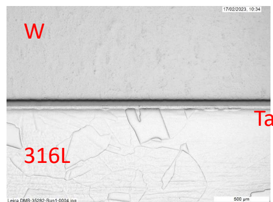
Figure 3 W-Ta-316L UDB joint with large grains in 316L substrate
