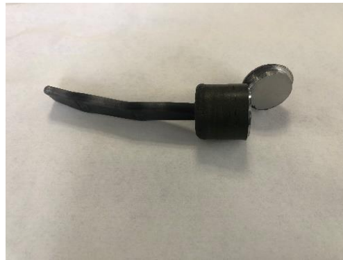
Figure 7 HIPed and machined cannister showing that the diffusion barrier successfully prevented bonding of 316L disc to
