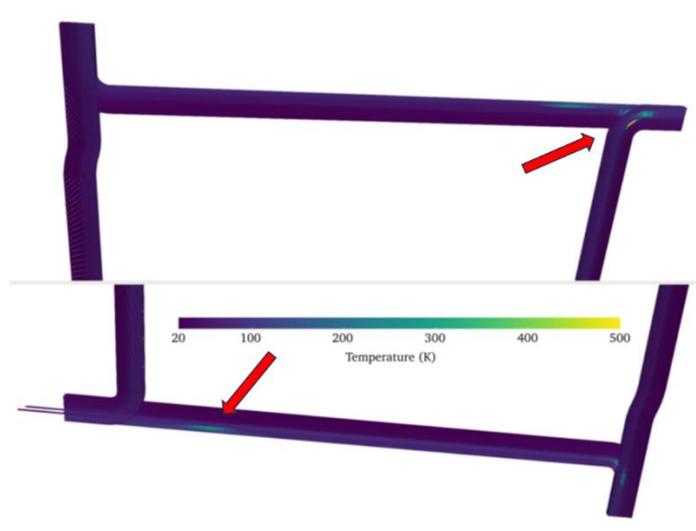
Figure 4: The temperature rises locally to 1000K in 300s, at which point the simulation is terminated.
