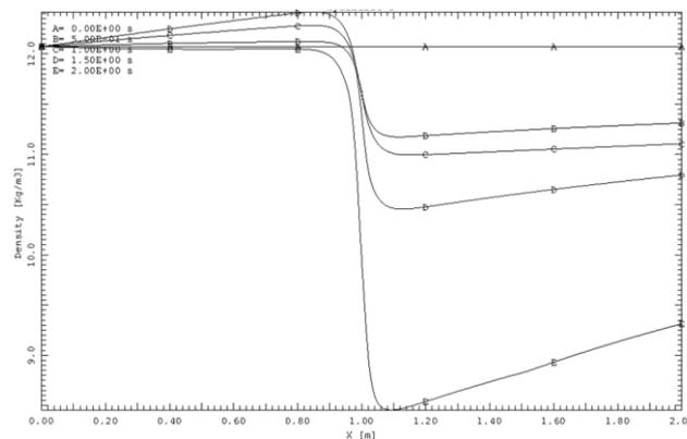
Figure 6: Helium coolant density along the quenching cable at various times.
