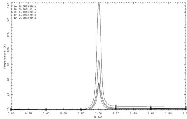
Figure 3: Temperature distribution along a cooled cable at various times after quench initiation.
