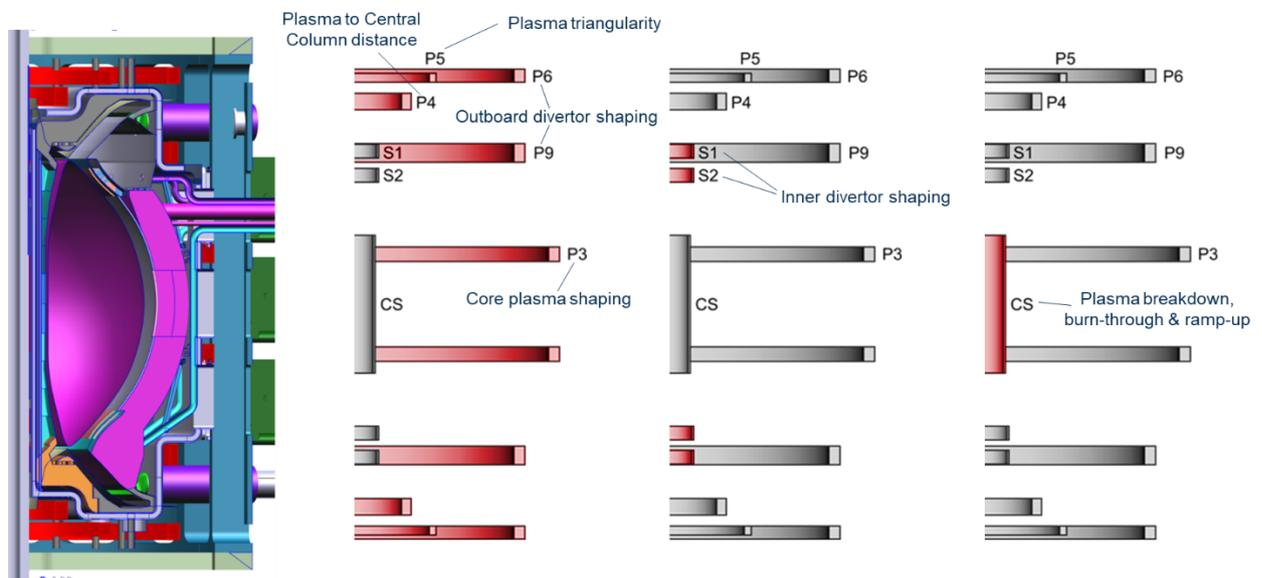
Figure 7: PF coil set and summary of plasma control functions.
