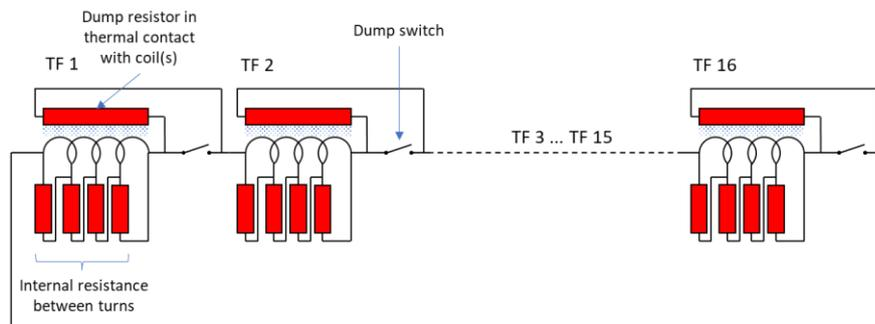
Figure 5: Dump switches are used to transfer stored magnet energy to heaters embedded in the coil structure.
