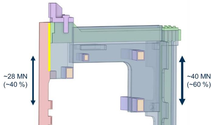
Figure 11: Force distribution through the inter coil structure.
