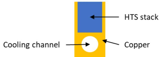
Figure 2: Cross section of a cable comprising a copper channel with a built-in cooling pipe and a simple stack of HTS tapes.
