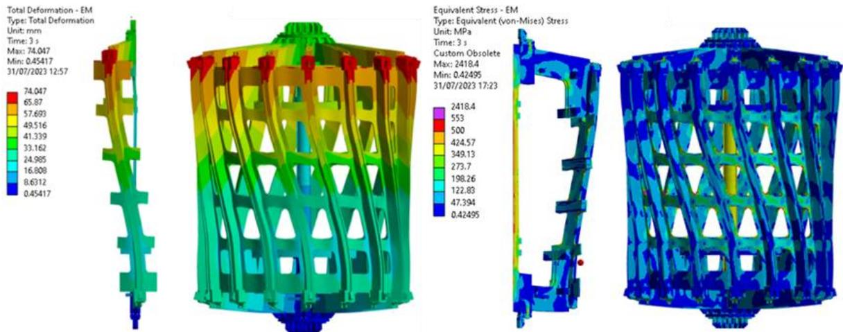
Figure 10: Total deformation plot and Von Mises stress plot under thermal and flat top EM loads.
