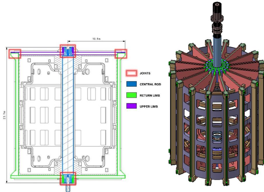
Figure 1: Cross section of the TF cage indicating segmentation of TF coil (left), and representation of the central rod being removed (right).
