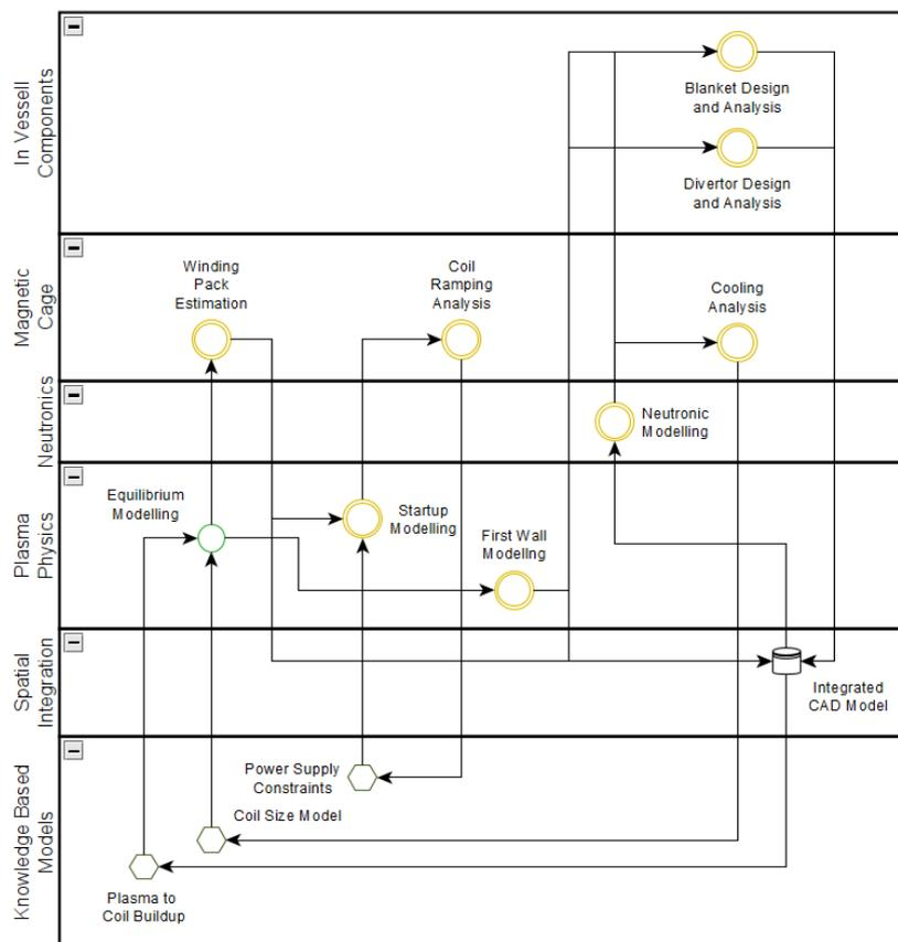
Figure 8: Simplified view of the design process.
