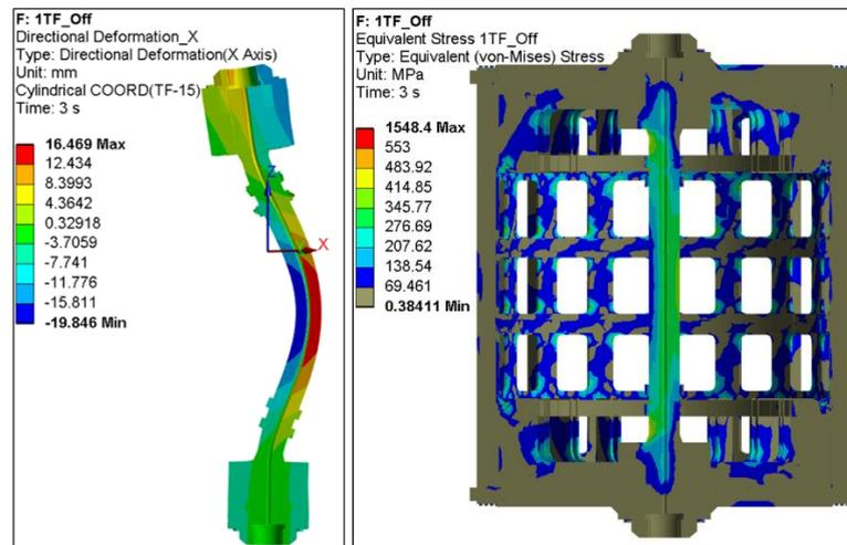
Figure 12: Fault load overview, (left) exaggerated radial deflection of central rod, (right) – stress plot of whole structure (cross-section through the centre of the machine).
