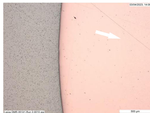
Fig. 4. A micrographic view of the sectioned diffusion bonding test run 2 sample. The CuCrZr/Cu bond region is indicated by the white arrow.
