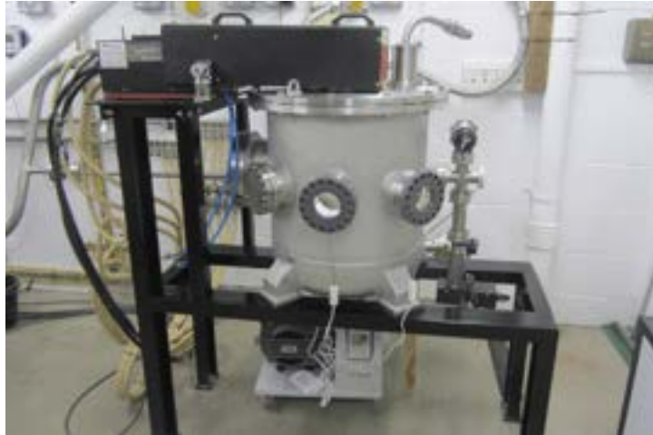
FIGURE 3.1: HIVE 's vacuum vessel (photo courtesy of UKAEA ).
